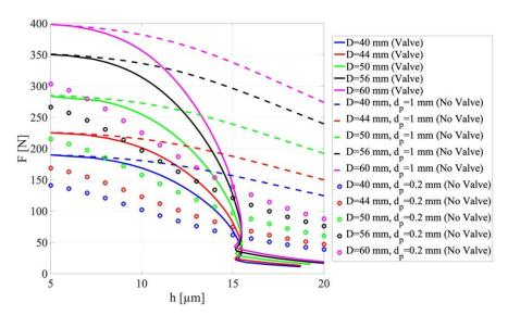
**Figure 16.** Comparison among the load capacities of the two benchmarks and compensated pad designed considering different outer diameters of the circular pad D, by considering the other parameters as constant:  $d_p = 1$  mm,  $d_v = 0.5$  mm,  $h^* = 15$   $\mu$ m and  $p_s = 0.7$  MPa.
