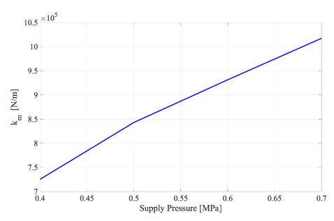
**Figure 21.** Trend of the optimal diaphragm stiffness expressed as a function of the supply pressure  $p_s$ , by considering the other parameters as constant:  $d_p = 1$  mm,  $d_v = 0.5$  mm,  $h^* = 15$   $\mu$ m and D = 40 mm.
