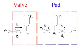
Figure 4. Lumped pneumatic circuit of the compensated pad.
