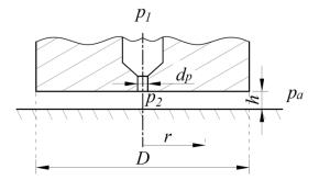
Figure 3. Scheme of the aerostatic pad.
