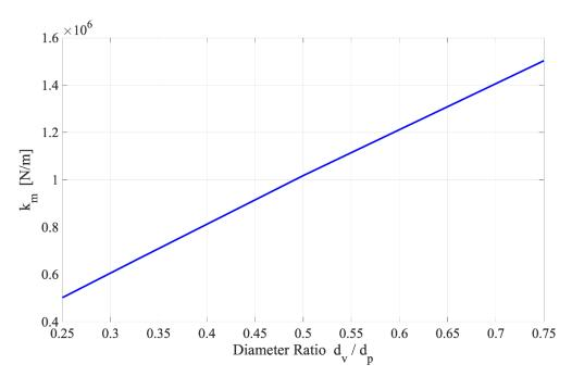
**Figure 15.** Trend of the optimal diaphragm stiffness expressed as a function of the diameter ratio  $d_v/d_p$  and orifice  $d_p$  diameters, by considering the other parameters as constant: D=40 mm,  $h^*=15$   $\mu$ m and  $p_s=0.7$  MPa.
