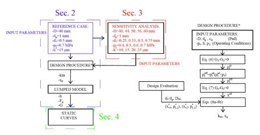
Figure 8. Flow charts summarizing the steps of the proposed design procedure and sensitivity analysis.
