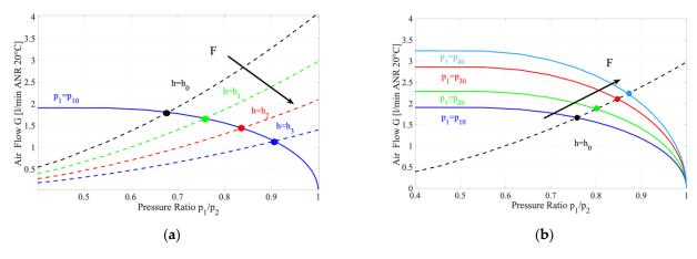
Figure 5. (a) Working conditions of a conventional pad. (b) Working conditions of a compensated pad.
