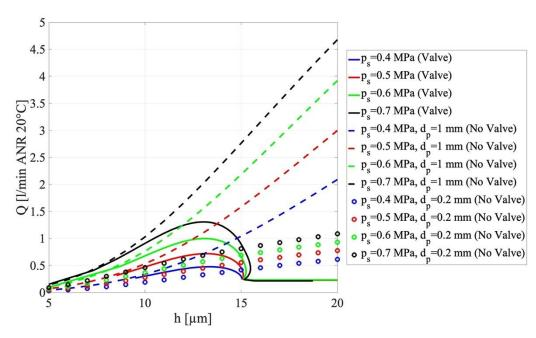
Figure 20. Comparison among the air consumptions of the two benchmarks and compensated pad designed considering different values of supply pressure  $p_s$ , by considering the other parameters as constant:  $d_p = 1$  mm,  $d_v = 0.5$  mm,  $h^* = 15$  μm and D = 40 mm.
