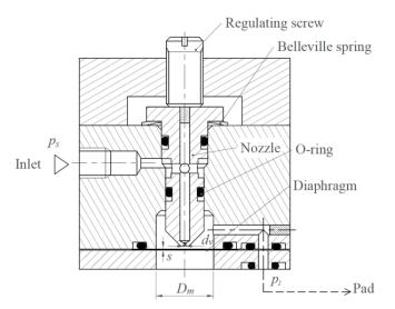
Figure 1. Scheme of the diaphragm valve.
