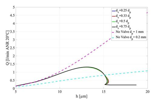
**Figure 14.** Comparison among the air consumptions of the two benchmarks and compensated pad designed considering different ratios of the nozzle  $d_v$  and orifice  $d_p$  diameters, by considering the other parameters as constant: D = 40 mm,  $h^* = 15$  µm and  $p_s = 0.7$  MPa.
