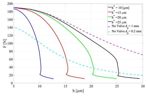
**Figure 9.** Comparison among the load capacities of the two benchmarks and compensated pad designed considering different desired air gap heights  $h^*$ , by considering the other parameters as constant: D = 40 mm,  $d_v = 1$  mm,  $d_v = 0.5$  mm and  $p_s = 0.7$  MPa.
