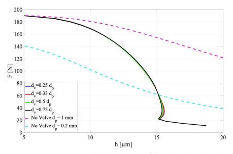
**Figure 13.** Comparison among the load capacities of the two benchmarks and compensated pad designed considering different ratios of the nozzle  $d_v$  diameters, by considering the other parameters as constant: D = 40 mm,  $h^* = 15$   $\mu$ m and  $p_s = 0.7$  MPa.
