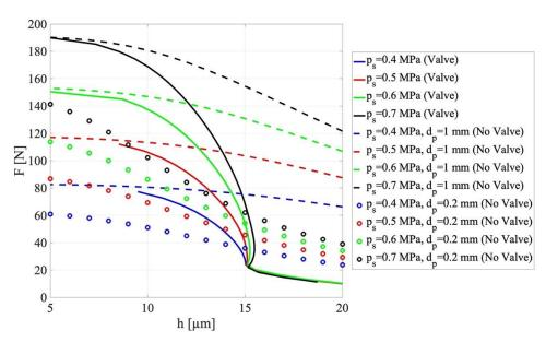
**Figure 19.** Comparison among the load capacities of the two benchmarks and compensated pad designed considering different values of the supply pressure  $p_s$ , by considering the other parameters as constant:  $d_p = 1$  mm,  $d_v = 0.5$  mm,  $h^* = 15$   $\mu$ m and D = 40 mm.
