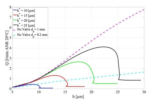
**Figure 10.** Comparison among the air consumptions of the two benchmarks and compensated pad designed considering different desired air gap heights  $h^*$ , by considering the other parameters as constant: D = 40 mm,  $d_p = 1$  mm,  $d_v = 0.5$  mm and  $p_s = 0.7$  MPa.
