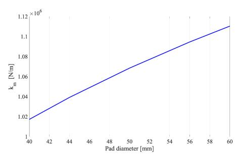
**Figure 18.** Trend of the optimal diaphragm stiffness expressed as a function of the outer diameter of the pad D, by considering the other parameters as constant:  $d_p = 1$  mm,  $d_v = 0.5$  mm,  $h^* = 15$   $\mu$ m and  $p_s = 0.7$  MPa.
