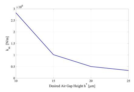
**Figure 11.** Trend of the optimal diaphragm stiffness expressed as a function of the desired air gap height  $h^*$ , by considering the other parameters as constant: D = 40 mm,  $d_p = 1$  mm,  $d_v = 0.5$  mm and  $p_s = 0.7$  MPa.
