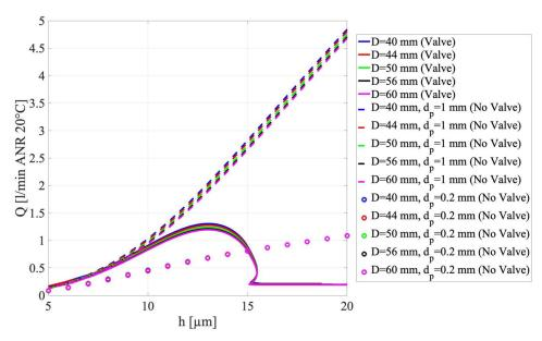
**Figure 17.** Comparison among air consumption of the two benchmarks and compensated pad designed considering different outer diameters of the circular pad D, by considering the other parameters as constant:  $d_p = 1$  mm,  $d_v = 0.5$  mm,  $h^* = 15$   $\mu$ m and  $p_s = 0.7$  MPa.
