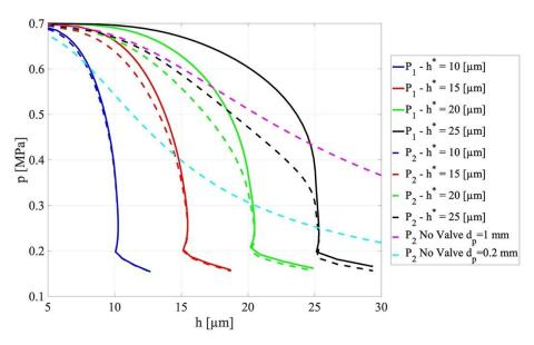
**Figure 12.** Comparison between the pressures upstream and downstream of the orifice of the pad considering different values of the desired air gap height  $h^*$ , by considering the other parameters as constant: D = 40 mm,  $d_v = 1$  mm,  $d_v = 0.5$  mm and  $p_s = 0.7$  MPa.
