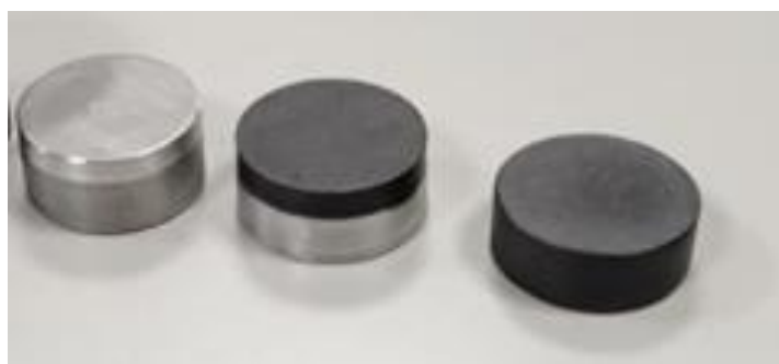
Figure 1. Samples for tribological characterization of the coating (from left to right: Babbitt metal, PEEK 101010, and PEEK cf15).
