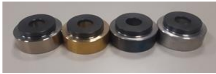
Figure 2. Samples with different backing metal (from left to right: 39CrNi, brass, aluminum, and AISI 304) with PEEK coating and geometry according to ISO 4386-2.
