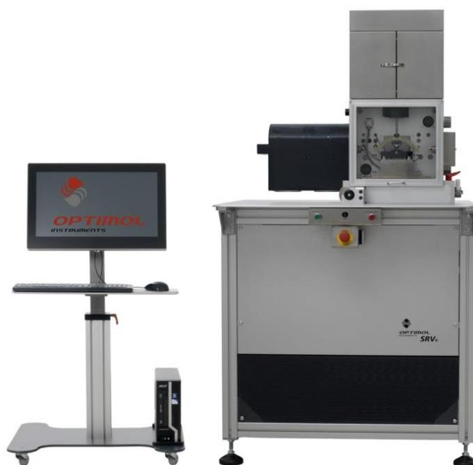
Figure 1. SRV model 5 tribometer with PC desk.
