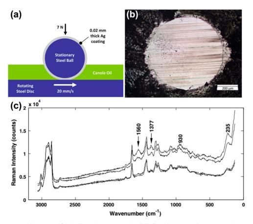
**Figure 4.** (a) Illustration of the ball-on-disc contact under fully flooded lubricated conditions. (b) Optical microscope image of the unwashed wear scar of the silver-coated ball for unrefined canola oil. (c) SERS spectra of the unwashed ball wear scar of refined canola oil with enhanced vibrational bands (labeled). (Adapted with permission from ref. [59]).
