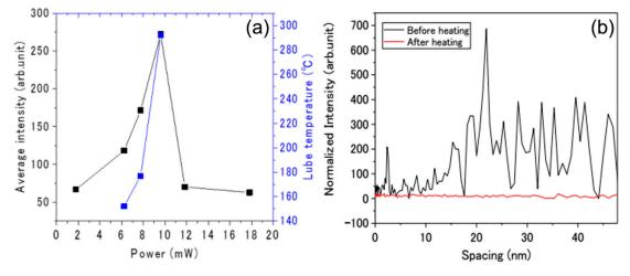
**Figure 7.** (a) Intensity change of the ether group and the temperature for lubricant film as a function of the laser power. (b) Intensity change of the ether group as a function of the spacing prior to and after laser heating. (Adapted with permission from ref. [75]).
