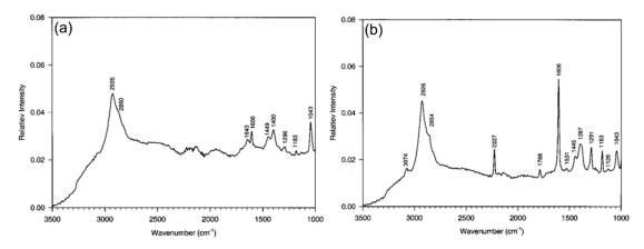
**Figure 8.** SERS spectrum of 6FDA-6CBBP from an unworn thin film contacted with a metallic layer. SERS spectrum of 6FDA-6CBBP from a worn thin film contacted with a metallic layer. (Adapted with permission from ref. [76]).
