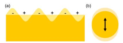
**Figure 1.** Schematic illustration of (**a**) surface plasmons and (**b**) a localized surface plasmon. (Adapted with permission from ref. [33]).
