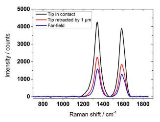
**Figure 3.** Comparison of three different tip-enhanced Raman spectra, all recorded with the same top-illuminating TERS setup but with a different tip distance. The probed material was a film consisting of carbon onions. All recorded spectra were baseline corrected. (Unpublished data of A. Rosenkranz).
