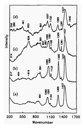
**Figure 5.** Raman spectra of (**a**) hexadecane on copper surface prior to rubbing, (**b**) after rubbing (100 m), (**c**) lubricated with hexadecane containing 0.4% stearic acid after rubbing for 100 m sliding distance, and (**d**) after 400 m sliding distance. (Adapted with permission from ref. [23]).
