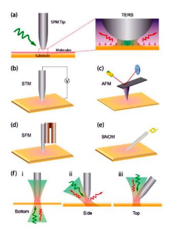
**Figure 2.** (a) Schematic illustration of different TERS setups using a STM (b), AFM (c), SFM (d), and SNOM (e). (f) Three different modes of excitation and collection need to be distinguished: (i) bottom excitation and collection, (ii) side excitation and collection, and (iii) top excitation and collection. (Adapted with permission from ref. [38]).
