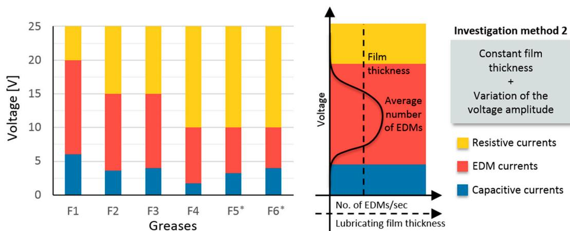
**Figure 8.** Measurement results of phase 2 with voltage variation (1–60 V). Determination of the capacitive, electric discharge machining (EDM) and resistive current ranges at steady-state temperature, a rotational speed of  $1000 \text{ min}^{-1}$ , an axial load of 200 N and an inverter switching frequency of 10 kHz (\* conductive greases).
