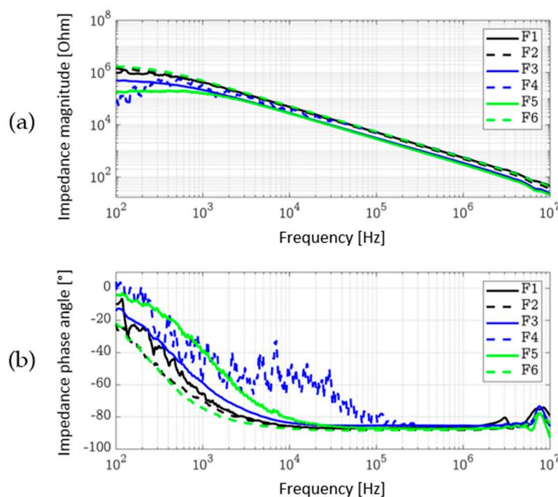
**Figure 7.** Measurement results of (a) the bearing impedance magnitude, and (b) the impedance phase angle after 16 h preconditioning at steady-state temperature, a rotational speed of  $1000 \text{ min}^{-1}$ , and a load of 200 N.
