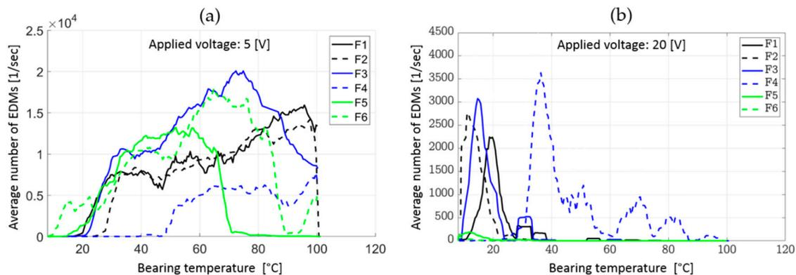
**Figure 9.** The average EDM breakdown number per second as a function of bearing temperature at a speed of  $1000 \text{ min}^{-1}$ , a load of 200 N and an inverter switching frequency of 10 kHz from phase 3 and 4 of the GESA investigations; (a) measurement results at an applied voltage of 5 V; (b) measurement results at an applied voltage of 20 V.
