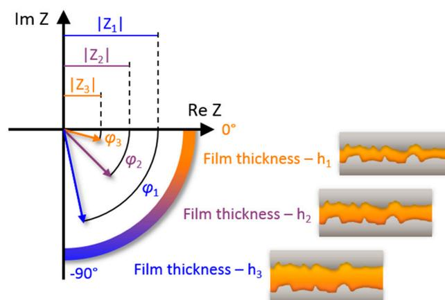
**Figure 2.** Relation between the lubrication film thickness and the complex impedance value.
