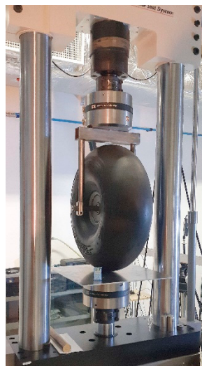
Figure 13. Vertical stiffness measurement test bench.
