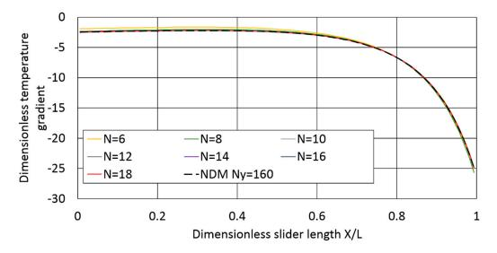
**Figure 10.** Dimensionless temperature gradient at the upper wall for the LPCM solution with imposed wall temperatures ( $h_1/h_2 = 4$ , Nx = 80 cells).
