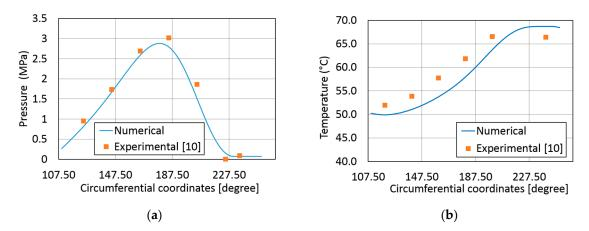
**Figure 22.** (a) Comparison of measured pressures and current numerical results in the mid plane of the loaded lobe (3500 rpm, 6 kN load), and (b) comparisons of measured temperatures and current numerical results in the mid plane of the loaded lobe.
