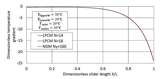
Figure 17. Dimensionless temperature gradient at the upper wall.
