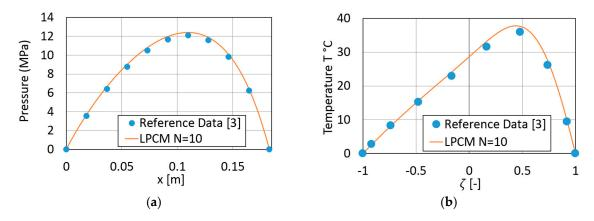
**Figure 19.** (a) Pressure variation in the 1D slider ( $h_1/h_2 = 2$ ) coupled thermo-hydrodynamic (THD) solution, and (b) outlet temperature variation across the film thickness in the 1D slider ( $h_1/h_2 = 2$ ) coupled THD solution.
