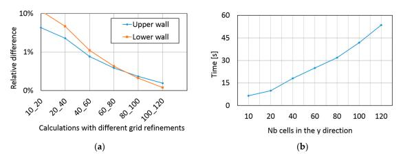
**Figure 20.** (a) Relative difference  $\varepsilon_K$  of the NDM for different grid refinements, and (b) computational time of the NDM for different numbers of cells, over the film thickness for the 1D THD slider.
