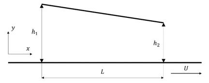
Figure 1. The 1D inclined slider.
