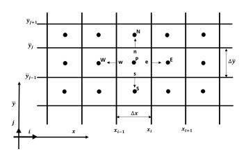
Figure 2. A typical 2D computational cell and the notation used for a 2D grid.
