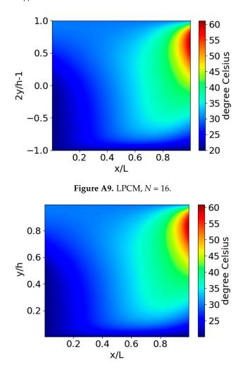
Case 5:  $h_1/h_2 = 4$ ,  $T_{UpperW} = 30 \,^{\circ}\text{C}$ ,  $T_{LowerW} = 20 \,^{\circ}\text{C}$ ,  $T_{inlet} = 20 \,^{\circ}\text{C}$ ,  $T_{outlet} = 20 \,^{\circ}\text{C}$ .
