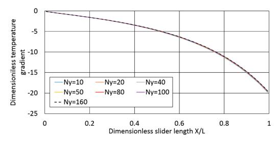
**Figure 4.** Dimensionless temperature gradient at the upper wall for the NDM solution and imposed wall temperatures ( $h_1/h_2 = 2$ , Nx = 80 cells).
