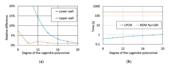
**Figure 14.** (a) Relative difference and (b) computational time of the LPCM solution for *Y* direction grid refinements ( $h_1/h_2 = 8$ , Nx = 80 cells).
