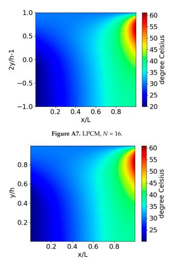
Case 4:  $h_1/h_2 = 4$ ,  $T_{UpperW} = 30 \ ^\circ\text{C}$ ,  $(\partial T/\partial y)_{LowerW} = 0$ ,  $T_{inlet} = 20 \ ^\circ\text{C}$ ,  $T_{outlet} = 20 \ ^\circ\text{C}$ .
