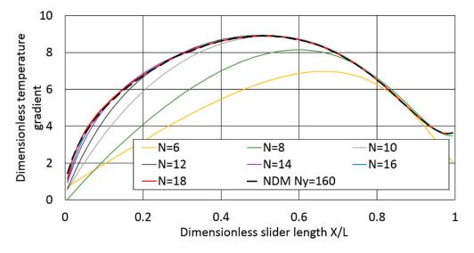
**Figure 9.** Dimensionless temperature gradient at the lower wall for the LPCM solution with imposed wall temperatures ( $h_1/h_2 = 4$ , Nx = 80 cells).
