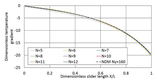
**Figure 7.** Dimensionless temperature gradient at the upper wall for the LPCM solution with imposed wall temperatures ( $h_1/h_2 = 2$ , Nx = 80 cells).
