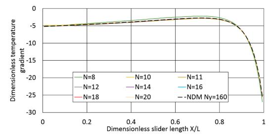
**Figure 13.** Dimensionless temperature gradient at the upper wall for the LPCM solution with imposed wall temperatures ( $h_1/h_2 = 8$ , Nx = 80 cells).
