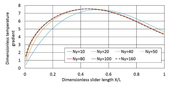
**Figure 3.** Dimensionless temperature gradient at the lower wall for the natural discretization method (NDM) solution and imposed wall temperatures ( $h_1/h_2 = 2$ , Nx = 80 cells).
