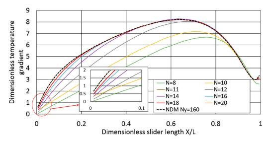
**Figure 12.** Dimensionless temperature gradient at the lower wall for the LPCM solution with imposed wall temperatures ( $h_1/h_2 = 8$ , Nx = 80 cells).
