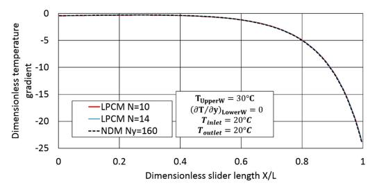
Figure 15. Dimensionless temperature gradient at the upper wall.
