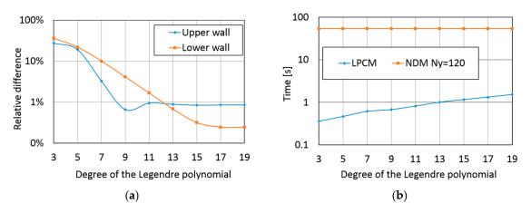
**Figure 21.** (a) Relative difference  $\varepsilon_N$  between the LPCM and the reference NDM Ny = 120, and (b) computational time of the LPCM compared to the reference NDM Ny = 120 results, for the 1D THD slider.
