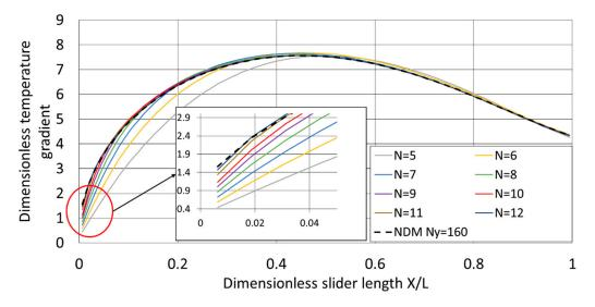
**Figure 6.** Dimensionless temperature gradient at the lower wall for the Lobatto Points Collocation Method (LPCM) solution with imposed wall temperatures ( $h_1/h_2 = 2$ , Nx = 80 cells).
