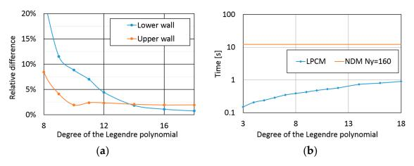
**Figure 11.** (a) Relative difference and (b) computational time of the LPCM solution for *Y* direction grid refinements ( $h_1/h_2 = 4$ , Nx = 80 cells).
