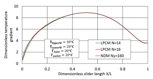
Figure 18. Dimensionless temperature gradient at the lower wall.
