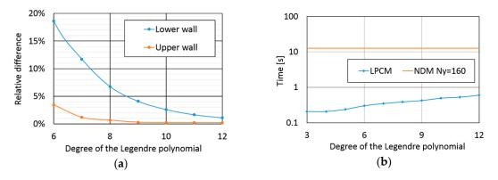
**Figure 8.** (a) Relative difference and (b) computational time of the LPCM solution for *Y* direction grid refinements ( $h_1/h_2 = 2$ , Nx = 80 cells)
