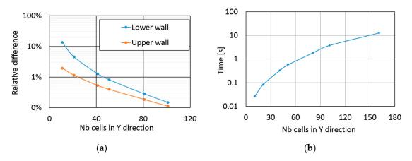
**Figure 5.** (a) Relative difference and (b) computational time of the NDM solution for *y* direction grid refinements ( $h_1/h_2 = 2$ , Nx = 80 cells).
