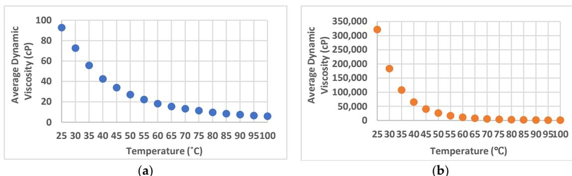
Figure 3. Viscosity of (a) mineral oil (MO) and (b) DCi.
