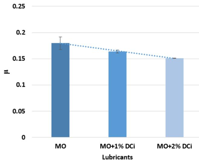
Figure 10. Average friction coefficient for a sliding velocity of 0.15 m/s.
