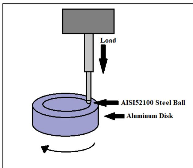
Figure 1. Pin-on-disk tribometer.
