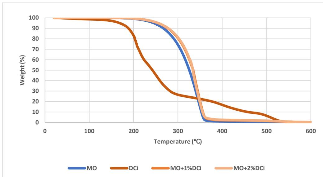
**Figure 4.** Experimental thermogravimetric analysis (TGA) for MO and DCi.
