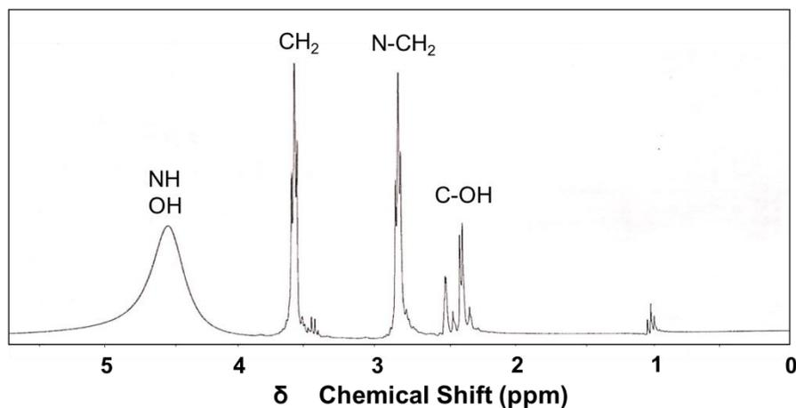
Figure 2. NMR spectrum of tri-[bis(2-hydroxyethylammonium)] citrate (DCi).
