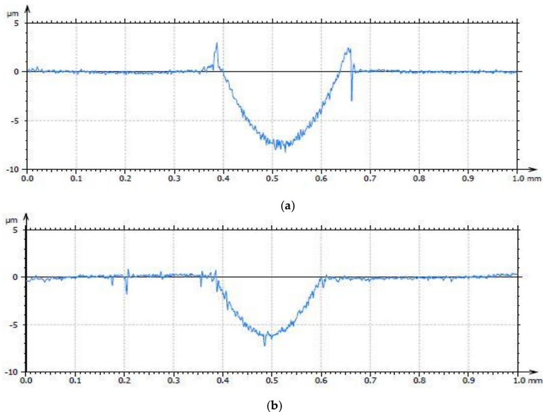
**Figure 15.** Two-dimensional (2D) profiles of wear tracks in tests with (a) MO, and (b) MO + 2% DCi.
