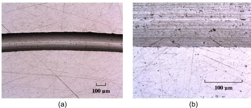
**Figure 13.** Wear track for a sliding velocity of 0.15 m/s: (a) MO + 2% DCi (50× magnification); (b) MO + 2% DCi (200× magnification).
