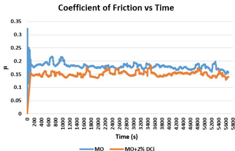
Figure 11. Friction coefficient vs. time when MO and MO + 2% DCi were used.
