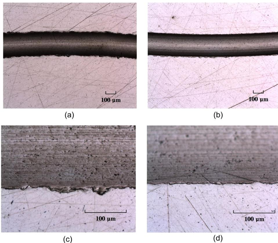
**Figure 7.** Wear tracks on aluminum discs for a sliding velocity of 0.10 m/s: (a,c) MO; (b,d) MO + 1% DCi. (a,b) Images are displayed with 50× magnification; (c,d) images are displayed with 200× magnification.
