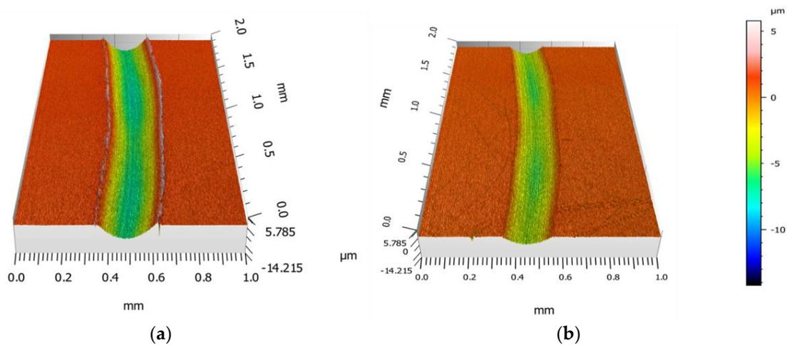
**Figure 14.** Three-dimensional (3D) profilometer images of wear tracks in tests with (a) MO, and (b) MO + 2% DCi.
