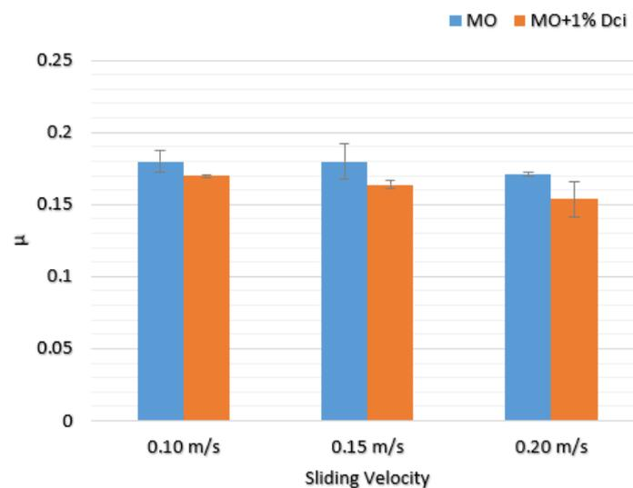
**Figure 5.** Average friction coefficients as a function of sliding velocity.
