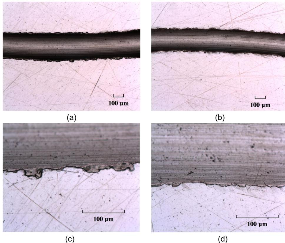
**Figure 8.** Wear tracks on aluminum discs for a sliding velocity of 0.15 m/s: (a,c) MO; (b,d) MO + 1% DCi. (a,b) Images are displayed with 50× magnification; (c,d) images are displayed with 200× magnification.
