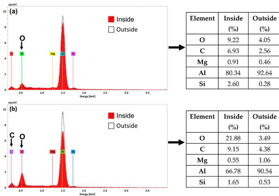
Figure 17. Energy-dispersive X-ray (EDX) spectrum of the inside and outside of the wear track with tables summarizing element percentages after tests lubricated with (a) MO, and (b) MO + 2% DCi.
