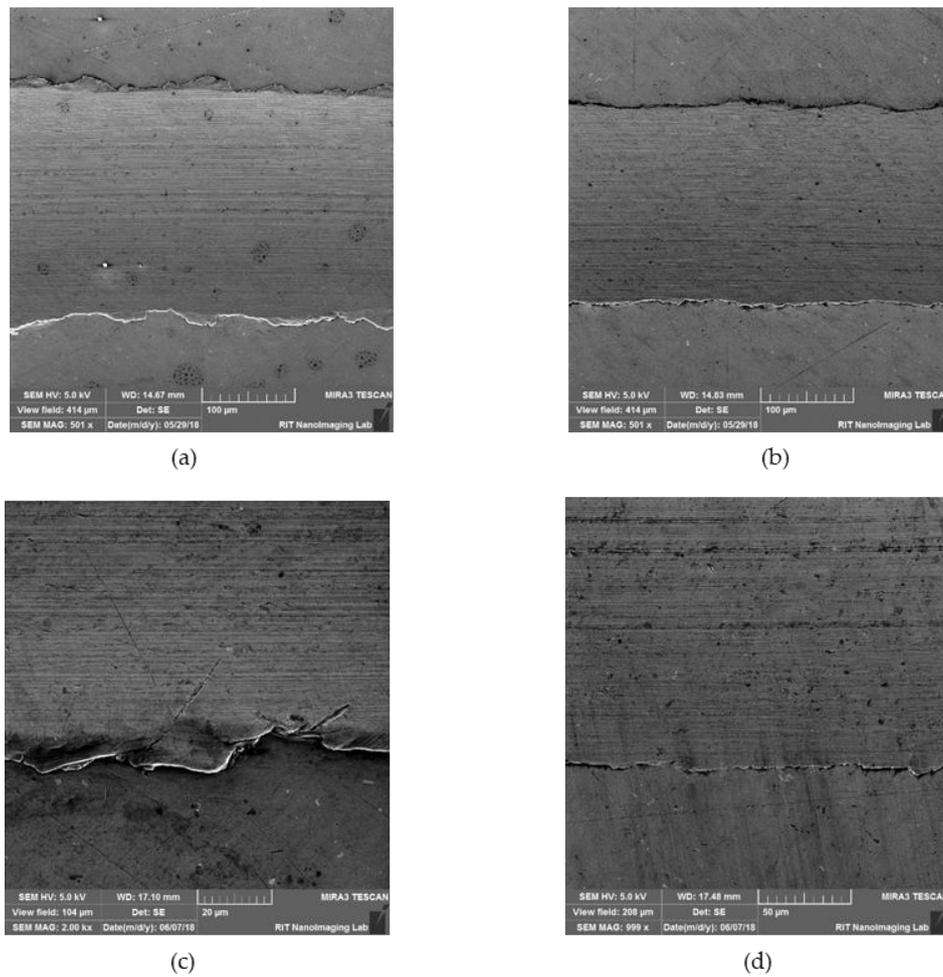
Figure 16. SEM micrographs for a sliding velocity of 0.15 m/s: (a,c) MO; (b,d) MO + 2% DCi.
