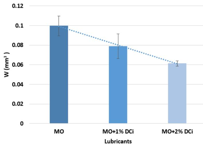
**Figure 12.** Loss of wear volume for different concentrations of ionic liquid at 0.15 m/s.
