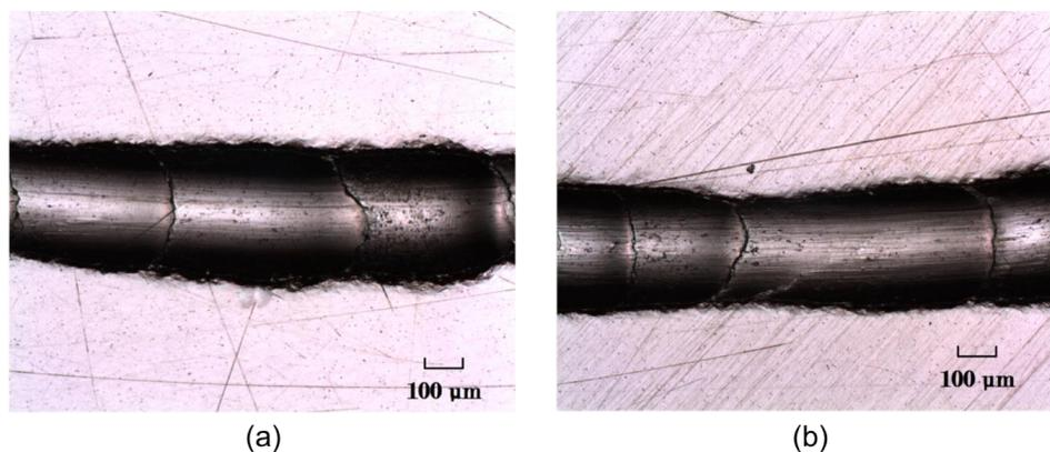
**Figure 9.** Wear tracks for a sliding velocity of 0.20 m/s: (a) MO; (b) MO + 1% DCi. Images are displayed with 50× magnification.
