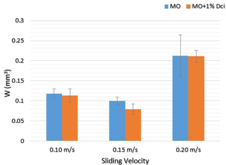
**Figure 6.** Wear volume on aluminum discs as a function of the sliding velocity.
