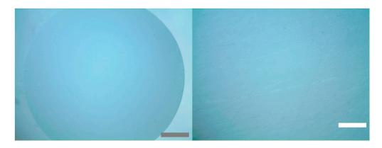
**Figure S1**. Optical microscopic images of UHWMPE pin (left) and disc (right) before tribological tests. The scale bars represent 1 mm.
