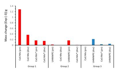
**Figure 4.** Mass changes in bearing materials after the tribological tests shown in Figures 2 and 3. Blue bars represent gains in the mass, and red bars represent losses in the mass.
