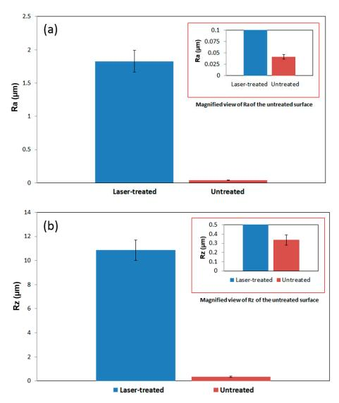
**Figure 8.** (a) Arithmetic mean deviation (Ra) and (b) maximum height (Rz) of the roughness profiles of the laser-treated and untreated CoCrMo surfaces (in Figure 7). The insets show the magnified view of Ra and Rz vs. of the untreated surface. The error bars indicated the standard deviation (SD) of n = 12.
