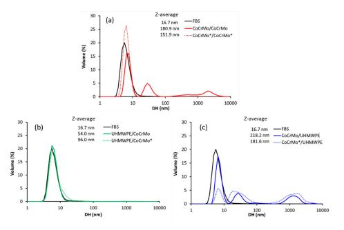
**Figure 6.** Distribution of hydrodynamic dimeter ( $D_H$ ) and Z-average values of FBS before and after tribological experiments with various tribopairs: (**a**) CoCrMo/CoCrMo and CoCrMo\*/CoCrMo\* pairs, (**b**) UHMWPE/CoCrMo and UHMWPE/CoCrMo\* pairs and (**c**) CoCrMo/UHMWPE and CoCrMo\*/UHMWPE pairs.
