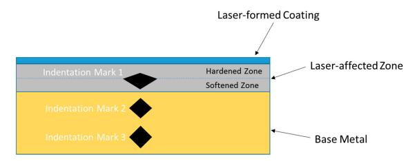
**Figure 10.** Graphical representation of the cross-section structure of the laser-treated CoCrMo surface. The laser-treated surface was composed of three different zones, namely laser-formed coating at the top, laser-affected zone in the middle, followed by the base metal at the bottom. The laser-affected zone can be sub-divided into the hardened zone (upper) and softened zone (lower).
