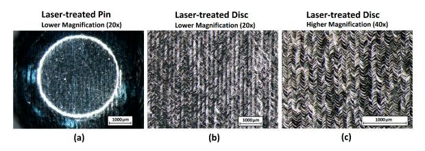
**Figure 1.** Optical micrograph image of laser-treated (**a**) pin  $(20 \times \text{magnification})$ , (**b**) disc  $(20 \times \text{magnification})$  and (**c**) disc  $(40 \times \text{magnification})$ .
