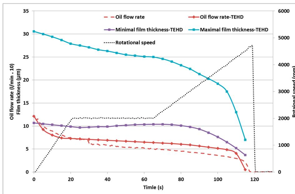
**Figure 13.** Comparison of the measured and simulated oil flow rate (increased by the factor of 10) and the shear losses (increased by the factor of 10) with the evolution of the simulated maximal and minimal film thicknesses.
