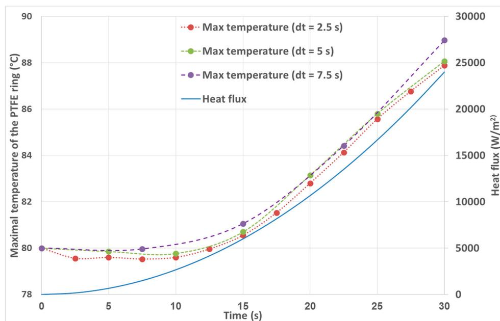
**Figure 6.** Preliminary pseudo-transient thermal analysis of the influence of time step on the geometry. The maximal temperature of the PTFE ring with three different time steps, while the heat flux is a pure parabolic function from 0 to  $24,000 \text{ W/m}^2$ , as a function of time.
