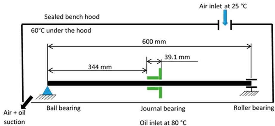
**Figure 2.** The test bench. The oil supply temperature of the bearing is 80 °C, while the air supply temperature is 25 °C, resulting in a 60 °C equilibrium temperature under the closed hood of the bench.
