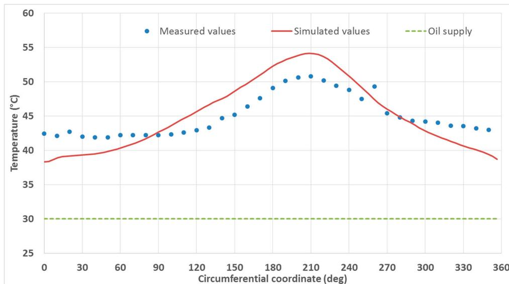
**Figure 11.** Simulated (TEHD) and measured temperatures [21] in the mid-plane (26.5 mm from the end) of the journal bearing, inside the groove.
