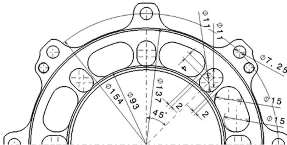
Figure 4. The detailed geometry of the symmetrical bushing.
