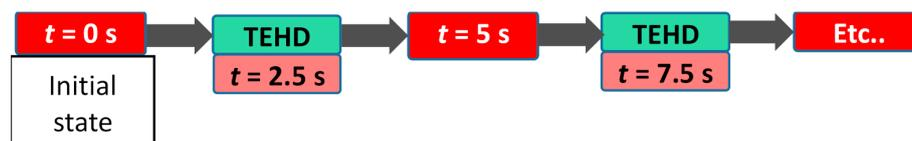
**Figure 7.** The pseudo-transient TEHD simulation flow chart. One TEHD simulation is executed for each 5 s interval, at the mid-point of each time step. After the convergence of one TEHD simulation, the thermal initial condition is updated and a new TEHD simulation is conducted with a new shaft rotational speed and heat convection coefficients.
