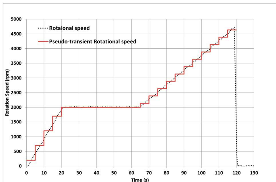
**Figure 8.** The start-up phase of the experiment is divided into 5 s long intervals for the transient TEHD simulation. The rotational speed of the shaft is constant and equal to the mean rotational speed of the shaft during each interval.
