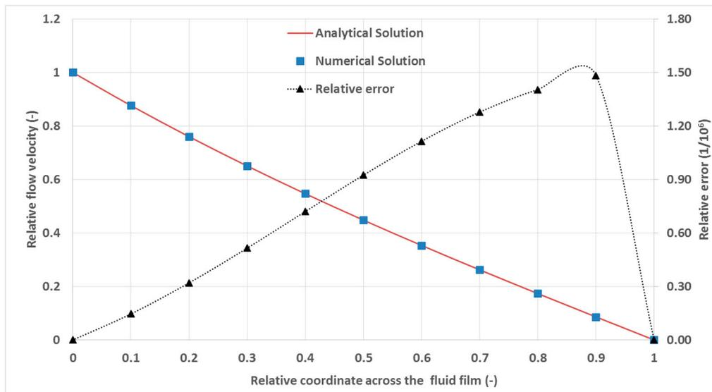
**Figure A2.** Comparison of the relativized numerical and analytical results. The analysed case was:  $h = 500 \mu\text{m}$ ,  $a_0 = 0.2 \text{ m/s}^2$ ,  $\nu = 3 \times 10^{-6} \text{ m}^2/\text{s}$ , at  $t = 0.1 \text{ s}$ , the flow being at rest at  $t = 0 \text{ s}$ . For the numerical solution, the domain was divided into 10 equidistant intervals and the constant time step was  $\Delta t = 0.00005 \text{ s} = 50 \mu\text{s}$ .
