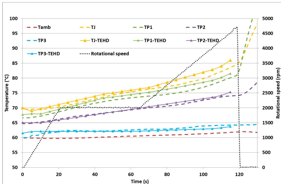
**Figure 12.** The temperature field at different locations of the bushing (simulated by the pseudo-transient TEHD model) compared to the measured values. Simulated values: continuous line (the triangles indicate each computational instance), measured values: dotted line.
