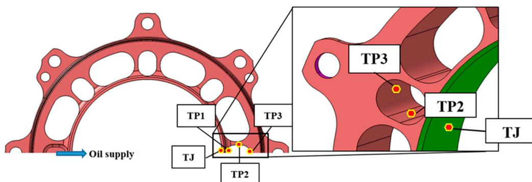
**Figure 3.** The symmetric steel bushing with the position of the thermocouples TP1, TP2, TP3 and TJ (each thermocouple is in the mid-plane of the journal bearing, TP3 is in cover on the zoomed view). The thermocouple TJ is in touch with the exterior of the PTFE ring, while TP1, TP2 and TP3 are in contact with the steel bushing, each being 180 degrees away from the oil supply entry position.
