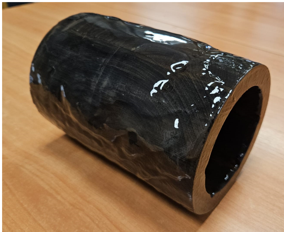
Figure 12. Substance formed on the bearing bush after two months of immersion in water.
