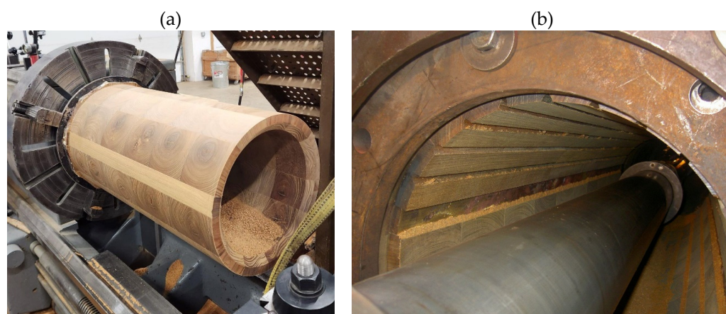
Figure 2. Manufacturing a wooden bearing bush: (a) a bush ready for installation during final turning; (b) machining of the bush after installation in the stern tube (authors' archive).
