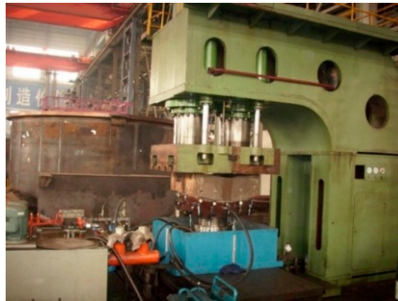
Figure 12. Single-shaft bearing sliding shoe bearing test apparatus.
