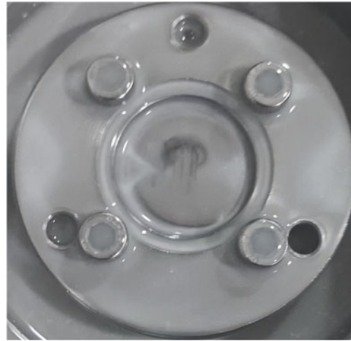
Figure 8. Before-cleaning optical image of the lower GCr15 specimen showing \text{Al}_2\text{O}_3 particles (white), mixed metal debris (black), and residual hydraulic oil after tribological testing at 10% abrasive concentration.
