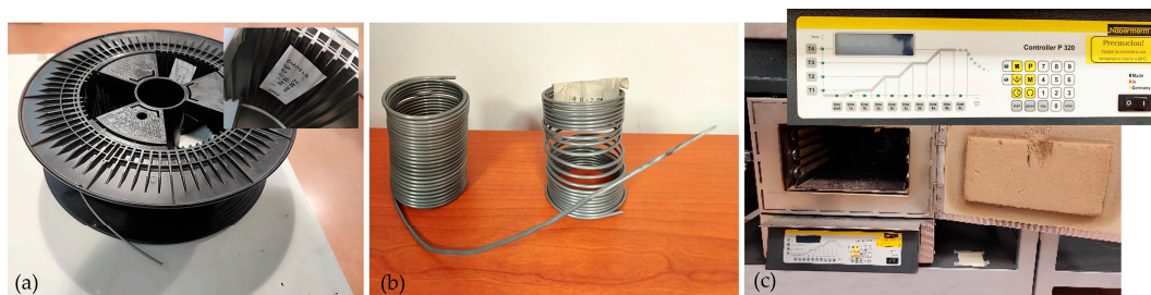
Figure 1. (a) ZnAl15% wire as supplied; (b) sample coils; and (c) Nabertherm N11/HR lab oven.
