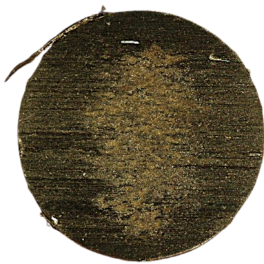
Figure 13. Details of wear in the pin with 1000 s, tested with texture sample and under lubricated conditions.
