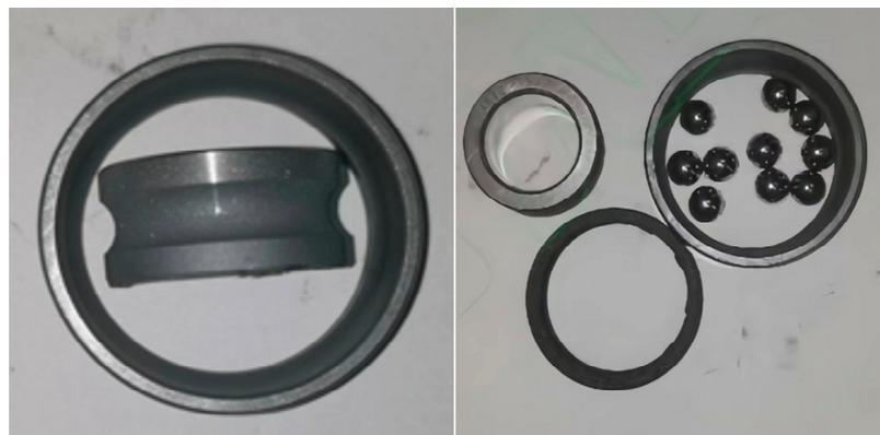
Figure 4. Bearing with MoS<sub>2</sub> coating.
