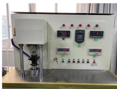
**Figure 14.** The HDM-20 end-face wear test machine.
