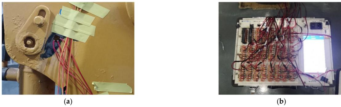
**Figure 6.** Experimental preparation process. (a) The strain gauge paste method. (b) The experiment preparation process.
