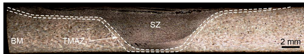
**Figure 8.** Cross-sectional view of the FSPed titanium sample at a distance of 5 mm from the start of the weld obtained using the ZhS32 tool.
