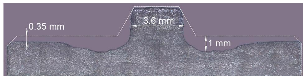
**Figure 4.** Axial cross-sectional view of the tool after traversing a distance of 2790 mm with a superimposed drawing of the initial tool geometry.
