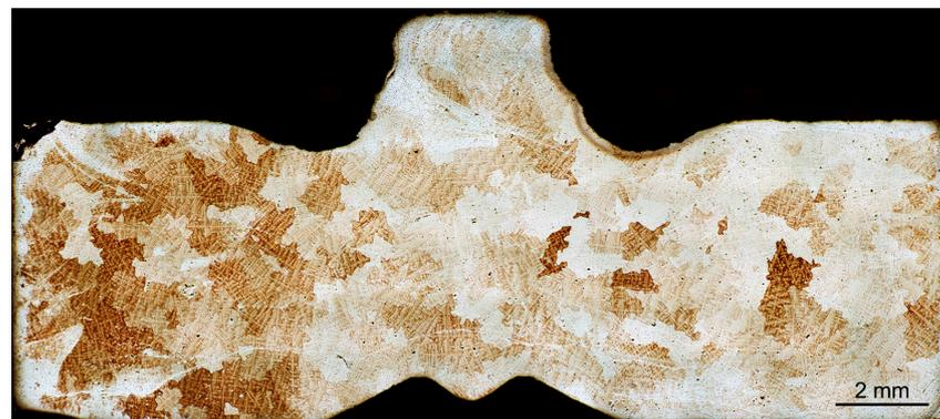
**Figure 14.** Axial cross-sectional metallographic image of the ZhS6U tool at a distance of 2790 mm from the start of friction stir processing with liquid cooling.
