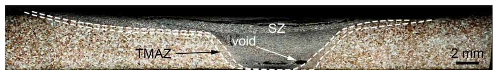
**Figure 9.** Cross-sectional view of the FSPed titanium sample at a distance of 240 mm from the start of the weld obtained using the ZhS32 tool.
