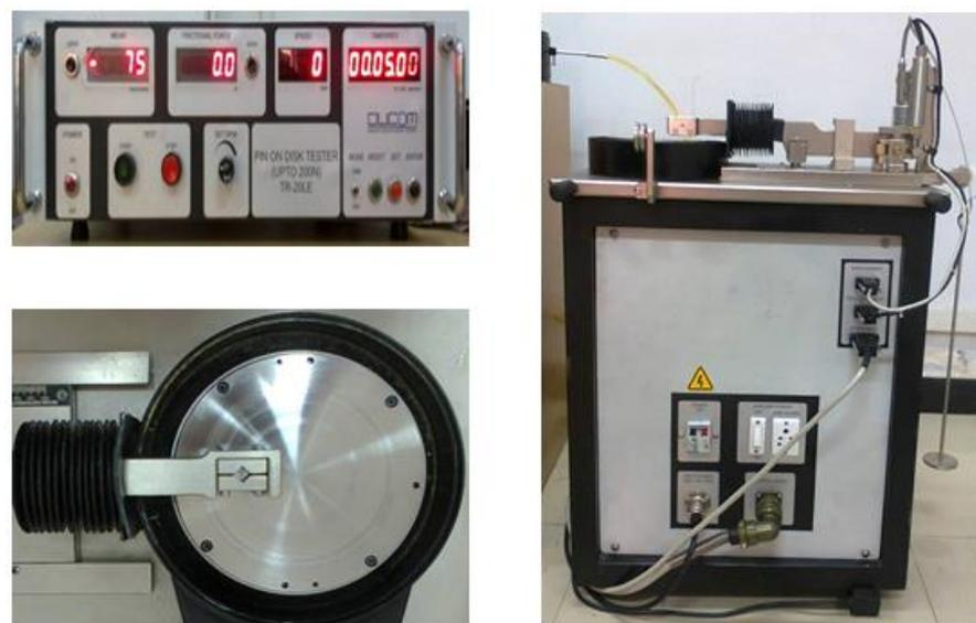
**Figure 1.** Wear test-Pin on disc.
