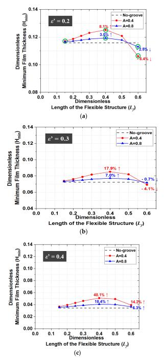
**Figure 11.** Dimensionless minimum film thickness with  $L_f$  (L = 3.0, W = 4.4,  $\gamma = 1.0$ ). (a)  $\varepsilon' = 0.2$ ; (b)  $\varepsilon' = 0.3$ ; (c)  $\varepsilon' = 0.4$ .
