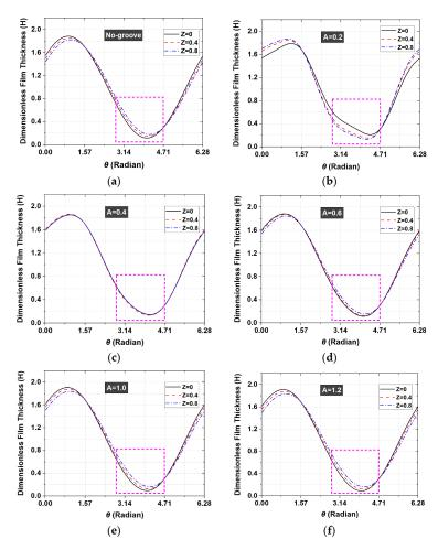
**Figure 10.** Circumferential distributions of the dimensionless film thickness for different A (L = 3.0,  $L_f$  = 1/3, W = 4.4,  $\gamma$  =1.0,  $\varepsilon'$  = 0.3). (a) No-groove; (b) A = 0.2; (c) A = 0.4; (d) A = 0.6; (e) A = 1.0; (f) A = 1.2.
