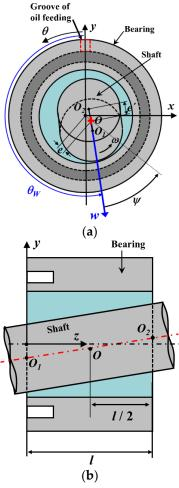
**Figure 3.** The shaft in the bearing with eccentric and tilted motion: (a) x-y plane; (b) y-z plane.
