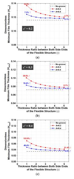
**Figure 14.** Dimensionless minimum film thickness with  $\gamma$  (L=3.0, W=4.4,  $\gamma=1.0$ ). (a)  $\varepsilon'=0.2$ ; (b)  $\varepsilon'=0.3$ ; (c)  $\varepsilon'=0.4$ .
