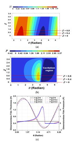
**Figure 6.** Dimensionless results for journal bearing without flexible structure (L = 3.0, W = 4.4,  $\gamma = 1.0$ ,  $\varepsilon' = 0.2$ ): (a) film thickness; (b) pressure distribution; (c) circumferential distribution of film thickness and pressure.
