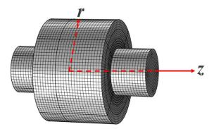
Figure 4. 3-dimensional finite element analysis model.
