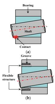
**Figure 1.** Application of the flexible structure to the misaligned journal bearing: (a) without flexible structure; (b) with flexible structure.
