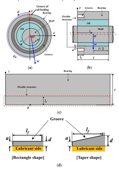
**Figure 2.** Schematics of the journal bearing system: (a) x-y plane; (b) y-z plane; (c)  $\theta-z$  plane; (d) shapes of the flexible structure.
