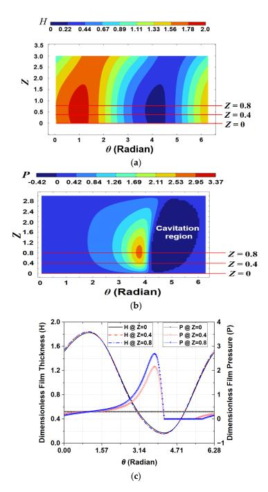
**Figure 7.** Dimensionless results for journal bearing with flexible structure (L = 3.0, A = 0.4, W = 4.4,  $\gamma = 1.0$ ,  $\varepsilon' = 0.2$ ): (a) film thickness; (b) pressure distribution; (c) circumferential distribution of film thickness and pressure.
