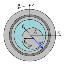
Figure 5. Oil film force working on the shaft.
