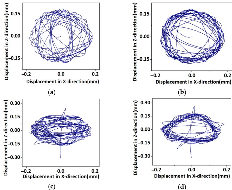
**Figure 17.** Radial axis displacement trajectory of eccentric  $0.05^\circ$  rotor under different axial protection clearance. (a) 0.1 mm Drop axis displacement; (b) 0.15 mm Drop axis displacement; (c) 0.2 mm Drop axis displacement; (d) 0.25 mm Drop axis displacement.
