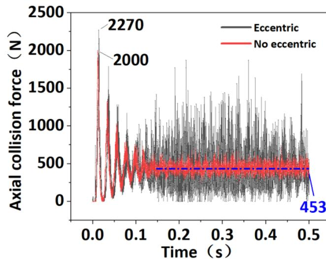
**Figure 6.** Comparison of the trend of the axial collision force at  $0.05^\circ$  with and without eccentricity.
