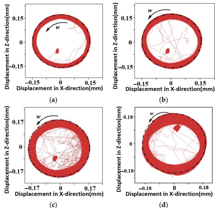
Figure 21. The centroid trajectory of rotors at different speeds in the process of falling collision. (a) 5 kr/min; (b) 10 kr/min; (c) 15 kr/min; (d) 20 kr/min.
