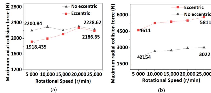
**Figure 15.** Comparison of maximum axial and radial collision forces under non-eccentric and eccentric working conditions. (a) Comparison of the maximum axial collision force of different speed rotor drops with eccentric  $0.05^\circ$ ; (b) Comparison of the maximum radial collision force of different quality rotor drops with the eccentric  $0.05^\circ$ .
