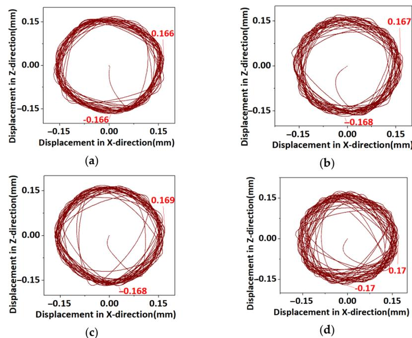
**Figure 16.** Radial axis displacement trajectory of the rotor under different axial protection gaps for non-eccentric working conditions. (a) 0.1 mm drop axis displacement; (b) 0.15 mm drop axis displacement; (c) 0.2 mm drop axis displacement; (d) 0.25 mm drop axis displacement.
