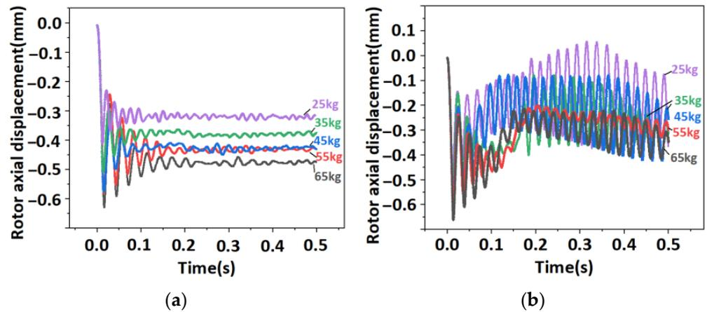
**Figure 8.** Comparison of non-eccentric and eccentric 0.05° rotor radial collision force. (a) Axial displacement of the rotor drops of different qualities under non-eccentric working conditions. (b) Axial displacement of rotor drops of different qualities at 0.05° eccentric conditions.
