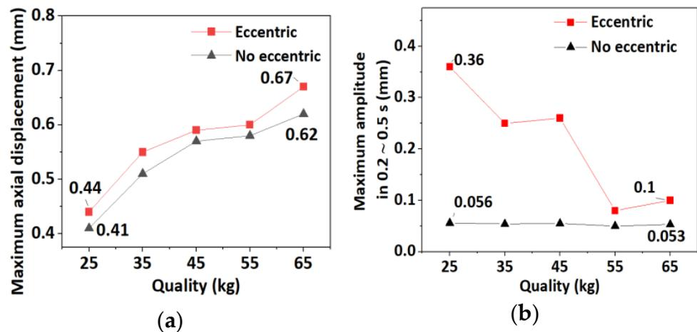
**Figure 9.** Comparison of maximum axial displacement and maximum amplitude of different quality rotor drops without eccentricity and eccentricity 0.05° working condition. (a) Comparison of the maximum axial displacement; (b) Comparison of the maximum amplitude within the 0.2~0.5 s.
