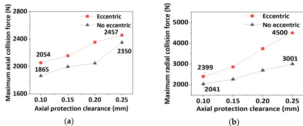
**Figure 19.** Comparison of maximum axial and radial collision forces under non-eccentric and eccentric working conditions. (a) Comparison of the maximum axial collision force of different axial protection clearance rotor drops under the  $0.05^\circ$  eccentric working condition; (b) Comparison of the maximum radial collision force of different axial protection gap rotor drops under the  $0.05^\circ$  eccentric working condition.
