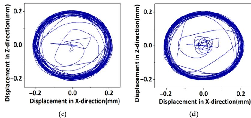
**Figure 12.** Radial displacement trajectory of non-eccentric and eccentric rotor shaft centers at different speeds. (a) 5000 r non-eccentric drop axis displacement; (b) 25,000 r non-eccentric drop axis displacement; (c) 5000 r eccentric 0.05° drop axis displacement; (d) 25,000 r eccentric 0.05° drop axis displacement.
