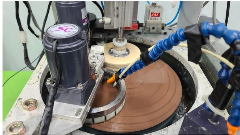
**Figure 1.** DMP machine used for SiC wafer preparation.
