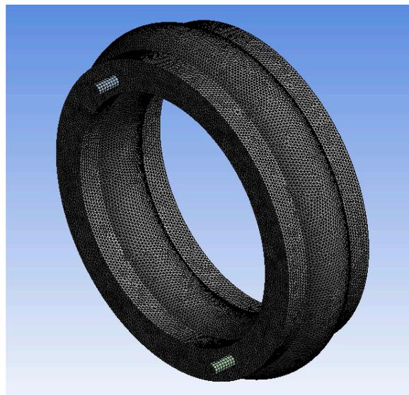
**Figure 8.** Bearing cavity grid.
