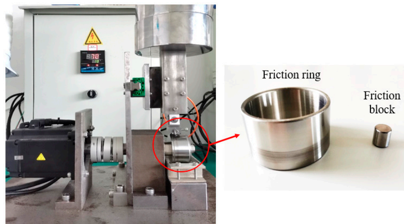
Figure 4. Ring block friction and wear test rig.
