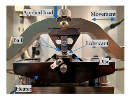
Figure 3. SRV assembly representation.
