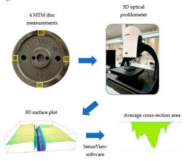
Figure 4. Wear measurement sequence.
