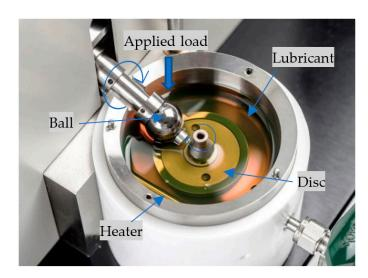
London, UK), represented in Figure 2. This apparatus is controlled with software which allows setting the load, the fluid temperature and the ball and disc rotational speeds.
