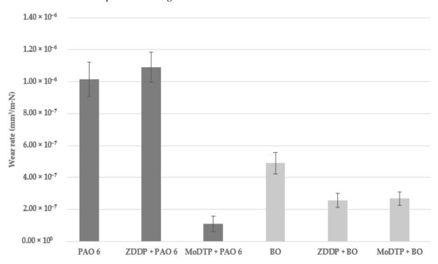
After the sliding/rolling test, the surface profilometries of the cleaned discs and balls, used with the final formulations, were completed. The overall average wear rates are represented in Figure 6.
