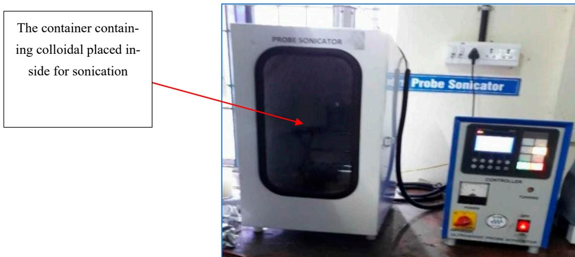
**Figure 2.** Probe sonicator setup used during the preparation of fluid.
