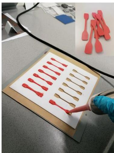
**Figure 1.** Preparation of adhesive dumbbell specimens according to EN ISO 527-2:2012.
