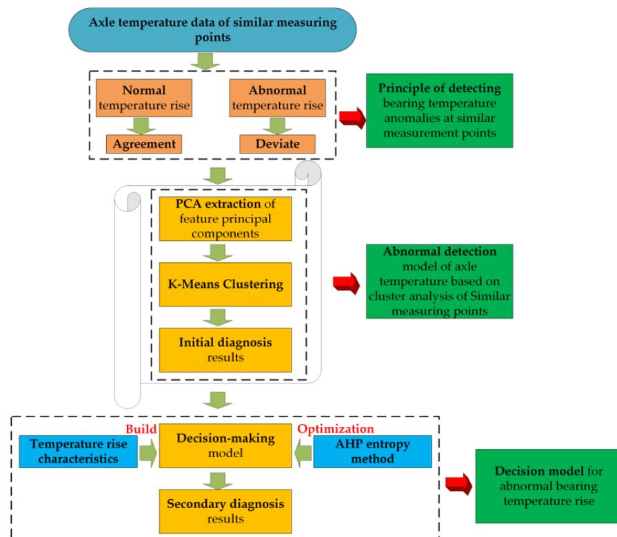
**Figure 18.** AHP-entropy-based model for detecting the abnormal temperature rise of the bearings [174].
