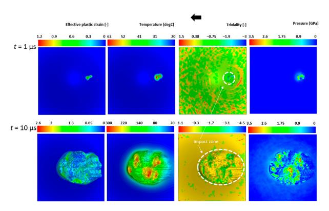
**Figure 14.** Top view of the strain, temperature, triaxiality and pressure results at two different time instances for Simulation C. The triaxiality result shows a larger dominance of shear stress around and inside the impact zone. The arrow shows the sliding direction.
