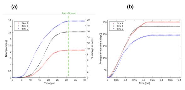
Figure 15. Worn mass of the lower body shown in (a) and average temperature in (b).
