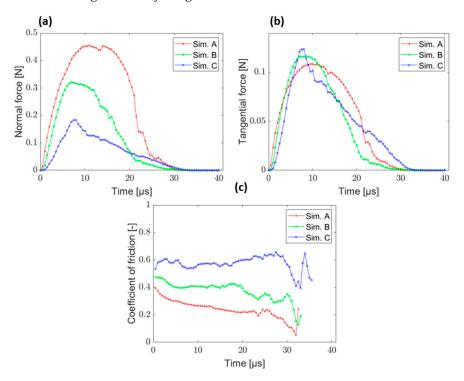
Figure 16. Normal force shown in (a), tangential force in (b) and the coefficient of friction in (c).
