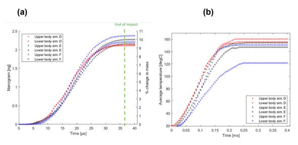
Figure 20. Worn mass of all bodies shown in (a) and average temperature in (b).
