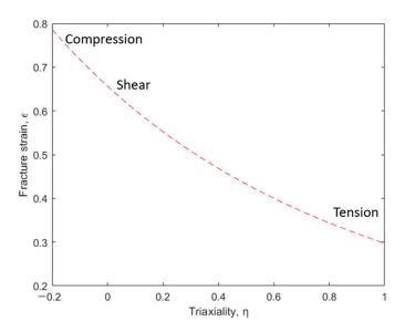
**Figure 9.** Fracture strain versus triaxiality for Lode parameter  $\overline{\theta} = 0$ .
