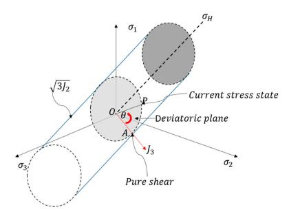
Figure 2. Illustration of the Lode angle in the principal stress space.
