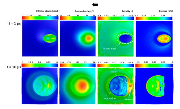
**Figure 13.** Top view of the strain, temperature, triaxiality and pressure results at two different time instances for Simulation A. The triaxiality shows all three stress states, i.e., compression (blue), shear and compression (green), pure shear (yellow) and tension (red). The arrow shows the sliding direction.
