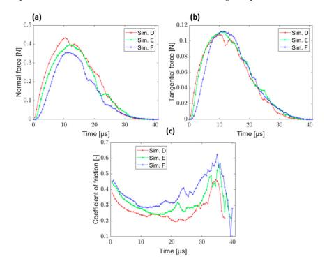
Figure 21. Normal force shown in (a), tangential force in (b) and the coefficient of friction in (c).
