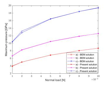
Figure 11. The maximum contact pressure for different normal loads and its comparison with BEM.
