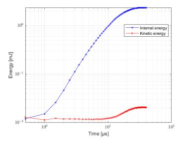
**Figure 26.** Internal strain energy and kinetic energy. The maximum kinetic energy reached is approximately 2% of the maximum reached internal energy.
