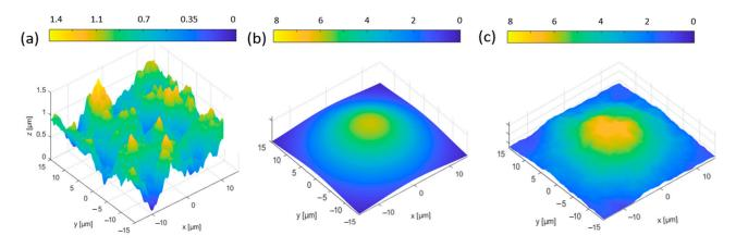
**Figure 6.** The figure shows the secondary roughness surface topography with an  $S_a$  value of 0.75 µm in (**a**), the smooth asperity in (**b**) and the final surface in (**c**) obtained after the surface in (**a**) is added to the surface in (**b**).
