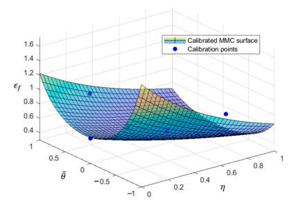
Figure 1. An example of the MMC surface calibrated for five different experiments [45].
