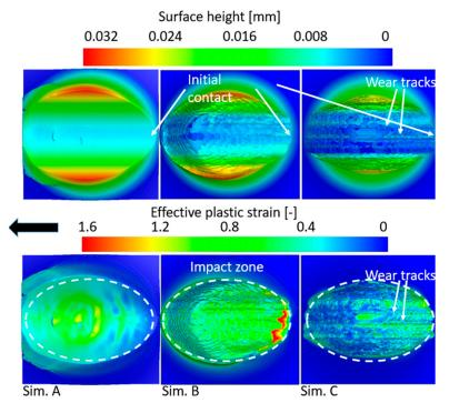
**Figure 18.** Top view of the surface height of the lower body for all three simulations at the end of impact, i.e.,  $t = 40 \ \mu s$  (**top**) and the final plastic strains (**bottom**). The impact zone is confined within the dashed area and the arrow shows the sliding direction of the upper body.
