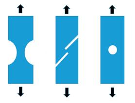
**Figure 3.** The figure shows the dog-bone specimen (**left**) for tension, simple shear specimen (**middle**) for shear and lastly the notched specimen (**right**) for combination of shear and tension.
