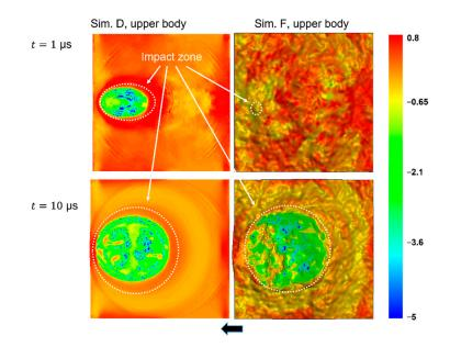
**Figure 22.** Top view of the triaxiality result for the upper bodes of Simulation D and F in Case 2. The stress states are dissimilar during initial contact as seen in the upper figures. The differences, however, fade with time as the upper body deforms and loses its sharp peaks during impact, as shown in the lower figures.
