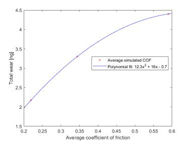
Figure 17. The average simulated COF together with a polynomial fit.
