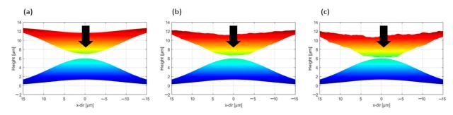
**Figure 10.** Simulations used to compare the present solution with BEM. A normal load is applied and the bodies are assumed to be linear elastic. Surface 1, 2 and 3 are used for the upper surfaces and shown in (**a**–**c**), respectively. Surface 1 is used for the lower surface for all simulations.
