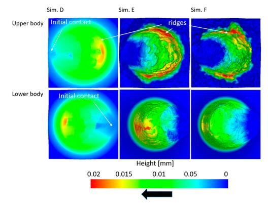
Figure 24. Final topographies of the bodies as viewed from the top and obtained at time 40  $\mu s.$
