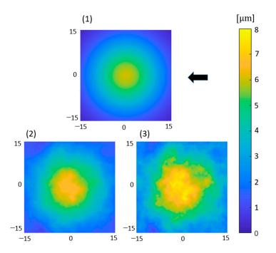
**Figure 7.** Top view of the final surface topographies used for the numerical experiments. Units are in  $\mu$ m and the arrow shows the sliding direction.
