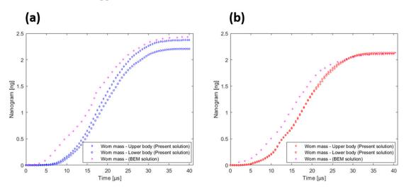
**Figure 27.** Comparison between the present solution and BEM for Sim. F shown in (**a**) and Sim. D shown in (**b**).
