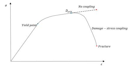
**Figure 4.** When the damage is coupled to stress at  $D = D_{crit}$ , the stresses are scaled back according to Equation (8) until D = 1 and fracture occurs.
