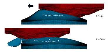
**Figure 12.** As the upper body moves, the lower body can be seen to plastically deform. The crack around the contact initializes and spreads quickly, causing abrasive wear on the lower body.
