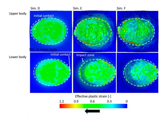
Figure 25. Effective plastic strain of all bodies as viewed from the top and at time 40  $\mu$ s.
