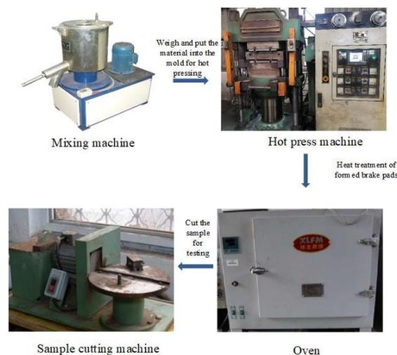
**Figure 3.** The preparation and sampling process of brake pad.
