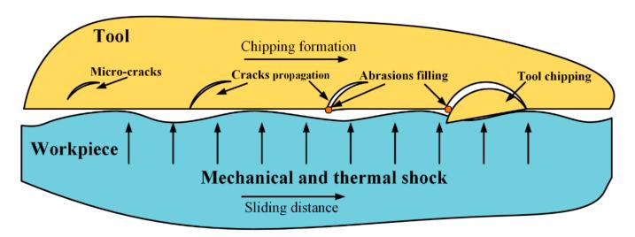
Figure 13. Tool chipping formation due to mechanical and thermal shock.
