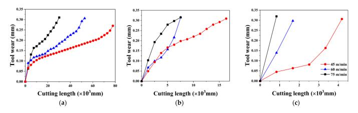
**Figure 6.** Tool wear progress curves at (a)  $f_z = 0.05 \text{ mm/r}$ , (b)  $f_z = 0.10 \text{ mm/r}$ , and (c)  $f_z = 0.15 \text{ mm/r}$ .
