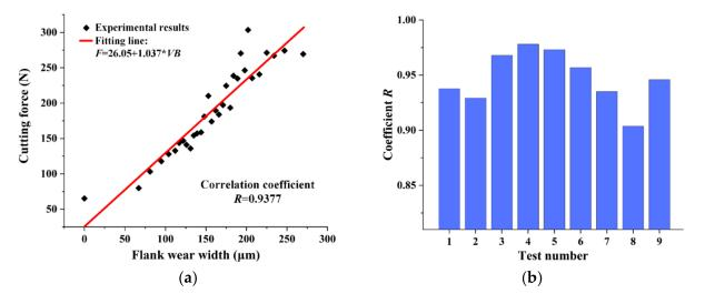
each test group are all over 0.9. This indicates that the tool wear and cutting force are linear in the milling process.
