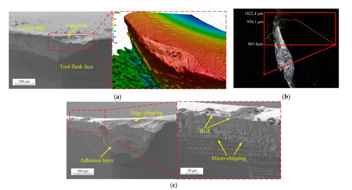
chippings caused by dramatic loads and the built-up edge appear on the flank face near the cutting edge. Traces of the adhesive layer and notching can be found on the flank face.
