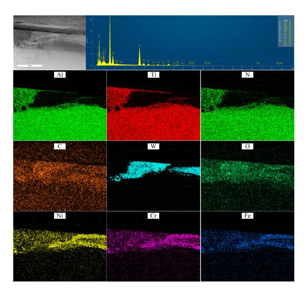
Figure 11. EDS mapping on tool worn flank face.
