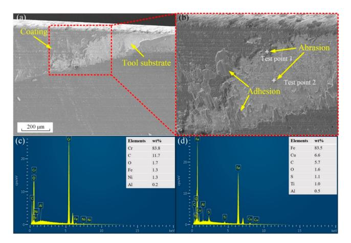
**Figure 8.** (**a**,**b**) Tool flank wear morphology at  $f_z = 0.05 \text{ mm/r}$  and  $v_c = 75 \text{ m/min}$  and (**c**,**d**) chemical compositions at Test point 1 and Test point 2, respectively.
