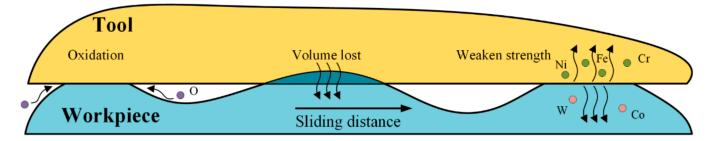
Figure 12. Tool wear progress with diffusion and oxidation.
