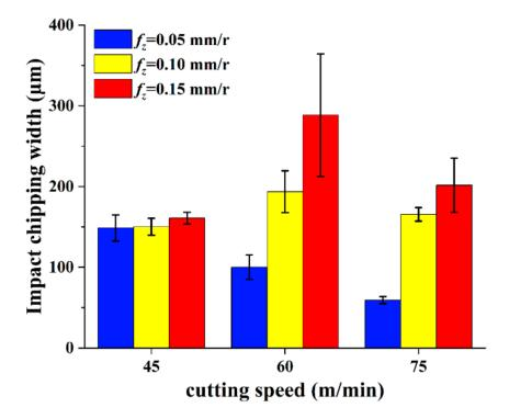
Figure 15. Tool chipping width at various cutting parameters.
