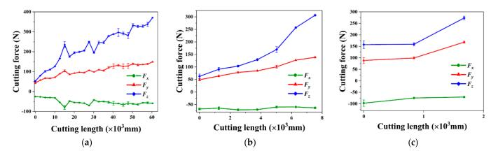
**Figure 4.** Cutting forces vs. cutting length at  $v_c = 60 \text{ m/min}$  and (a)  $f_z = 0.05 \text{ mm/r}$ , (b)  $f_z = 0.10 \text{ mm/r}$ , and (c)  $f_z = 0.15 \text{ mm/r}$ .
