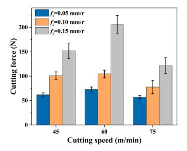
Figure 3. Cutting force at different cutting parameters with new inserts.
