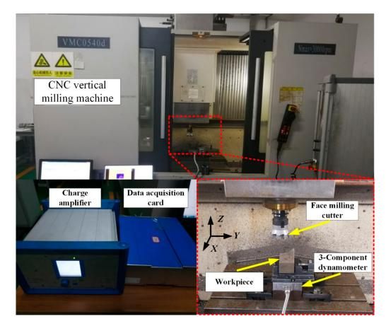
Figure 1. Face milling experiments.
