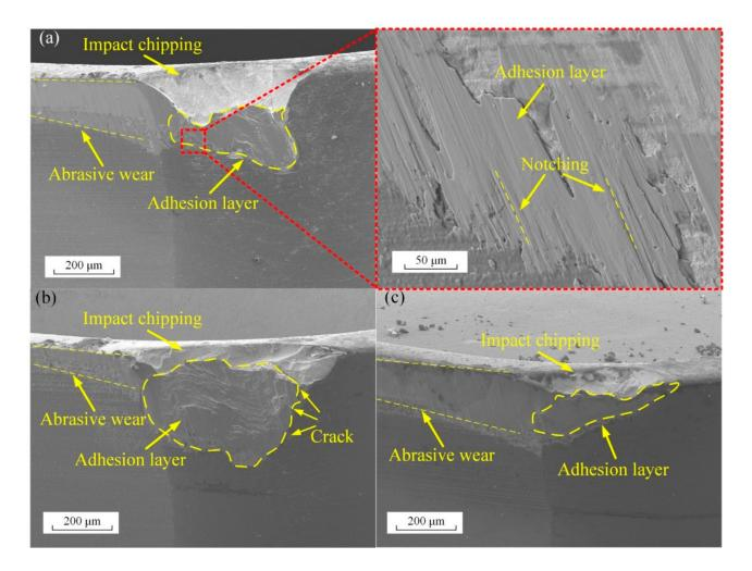
**Figure 10.** SEM images of Inconel 718 adhesion layer on tool surface at the cutting speed of (**a**) 45 m/min, (**b**) 60 m/min, and (**c**) 75 m/min.
