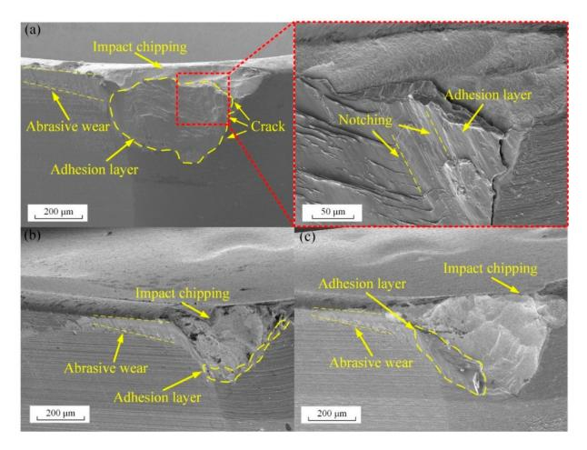
**Figure 9.** SEM images of Inconel 718 adhesion layer on tool surface at feed rate of (**a**) 0.05 mm/r, (**b**) 0.10 mm/r, and (**c**) 0.15 mm/r.
