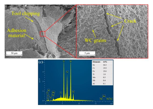
**Figure 14.** SEM image of micro-crack propagations under tool surface with (**a**) low and (**b**) high magnifications, and (**c**) EDS results of adhesion material.
