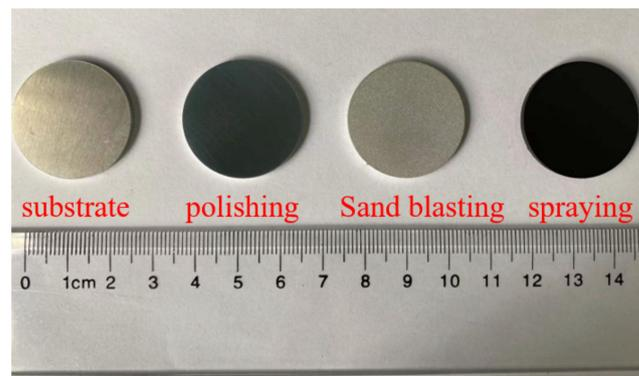
**Figure 1.** Specimen preparation process.
