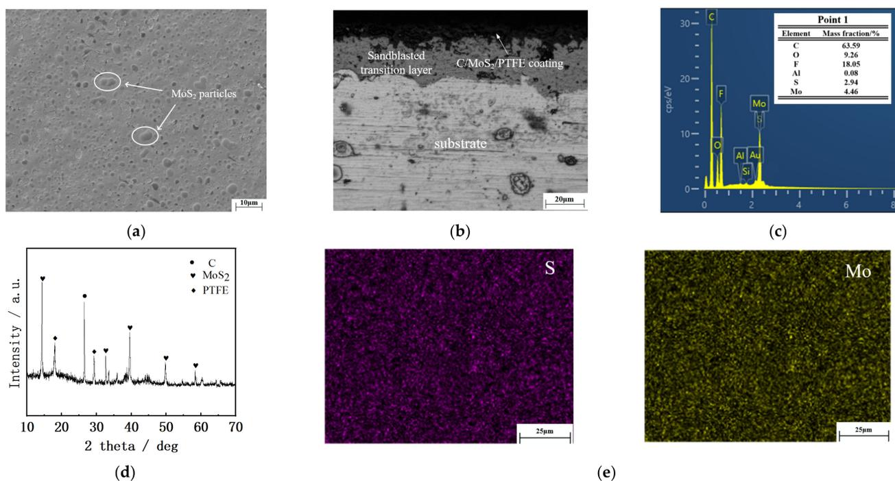
**Figure 3.** SEM morphology, surface XRD pattern, and EDS composition of C-MoS<sub>2</sub>-PTFE coating surface and OM morphology of coating cross-section. (a) SEM images of coated surfaces, (b) Optical microscopy of coating cross-section, (c) EDS analysis of coated surface, (d) XRD patterns of a Coated surface, (e) Element distribution diagram of coating material.
