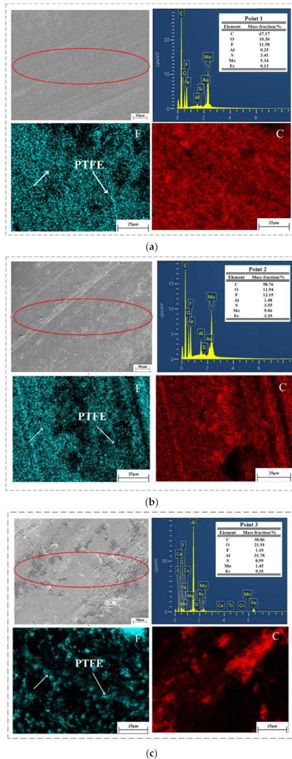
**Figure 8.** EDS surface scan image of surface wear of different loads modified C-MoS<sub>2</sub>-PTFE coating. (a) 5 N, (b) 10 N, (c) 15 N.
