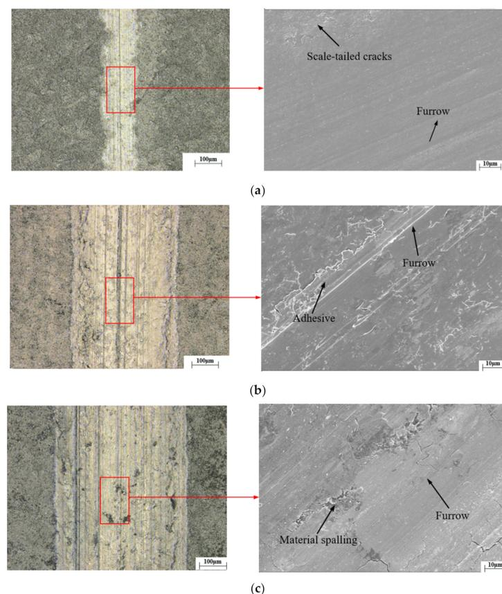
**Figure 7.** Worn surface morphology of C-MoS<sub>2</sub>-PTFE coating under different loads. (a) 5 N, (b) 10 N, (c) 15 N.
