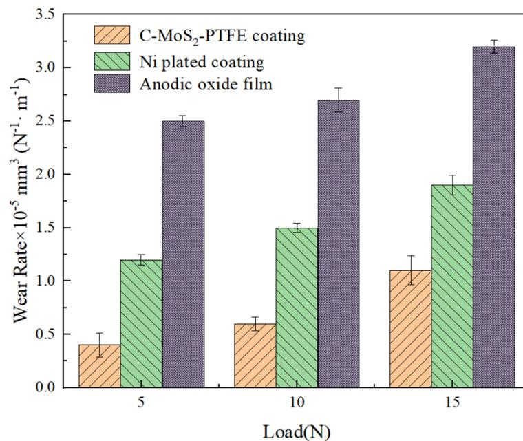
Figure 5. Wear rate under different loads.
