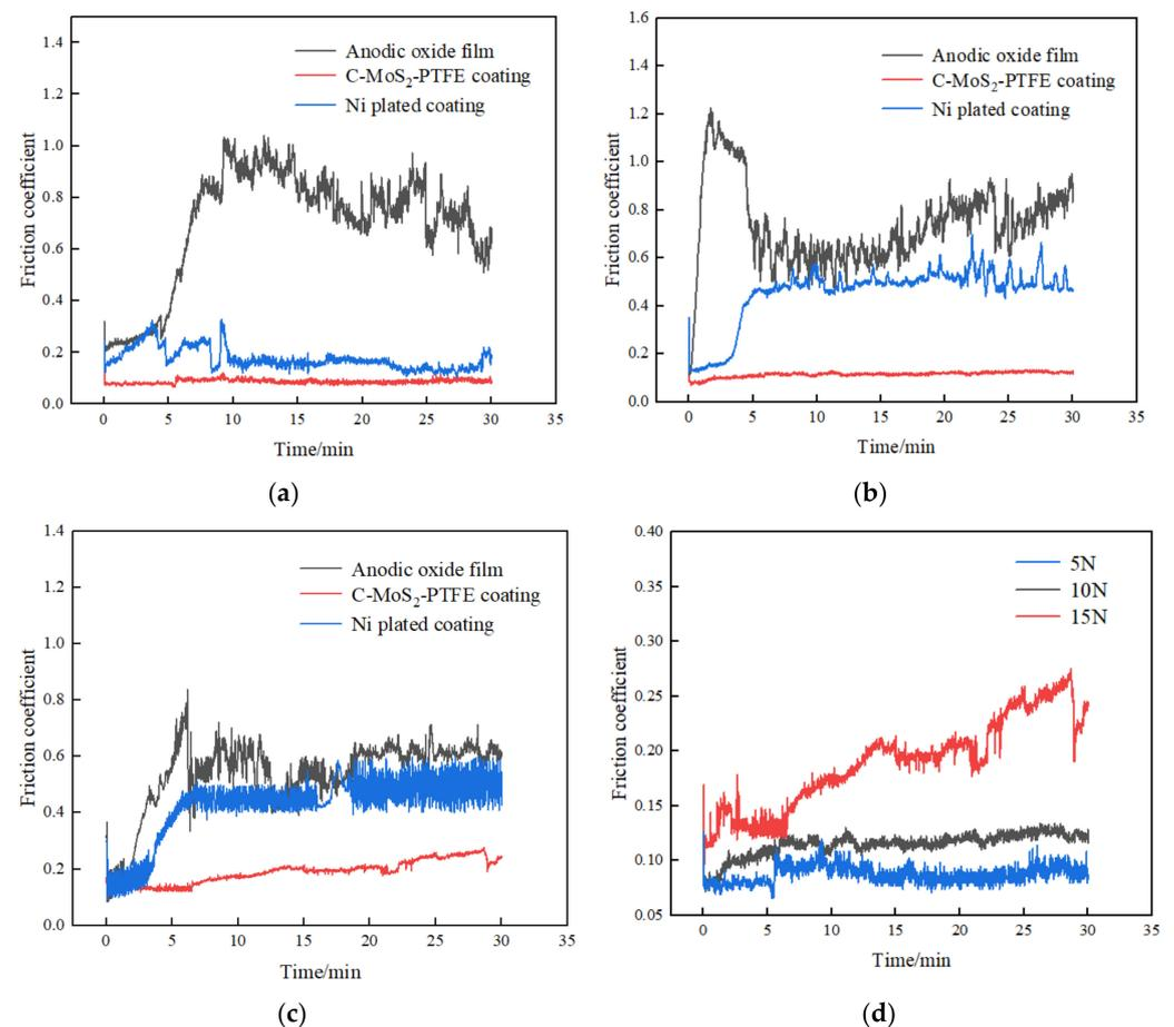
**Figure 4.** Friction coefficient under different loads. (a) 5 N, (b) 10 N, (c) 15 N, (d) Friction coefficient of C-MoS<sub>2</sub>-PTFE coating under different loads.
