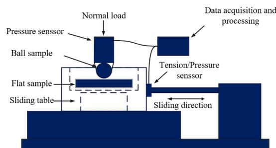
**Figure 2.** Structure diagram of reciprocating Friction and wear tester tribometer.
