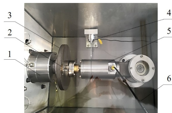
Figure 4. The internal structure of the test bench (1, mainshaft; 2, slipper assembly; 3, swashplate; 4, tension sensor; 5, piston assembly; 6, pressure oil circuit).
