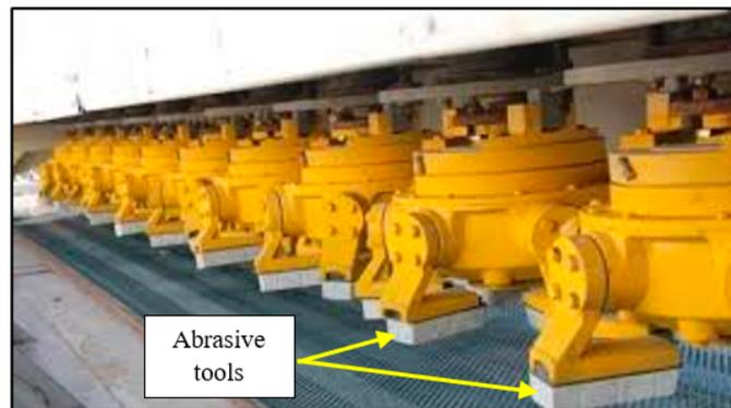
**Figure 1.** A long polishing machine with successive heads.
