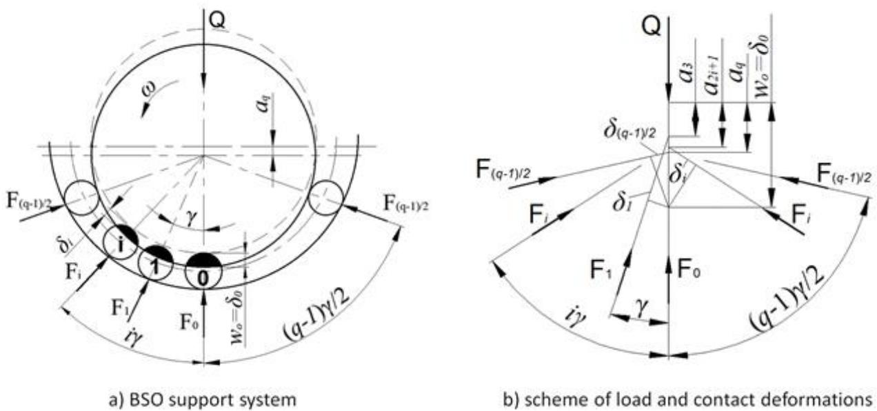
Figure 1. The internal radial load distribution in the *BSO* position of the rolling elements set.
