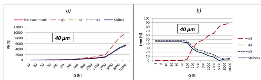
Figure 8. The radial ball bearing 6206 with an internal radial clearance  $e = 40 \mu\text{m}$ .
