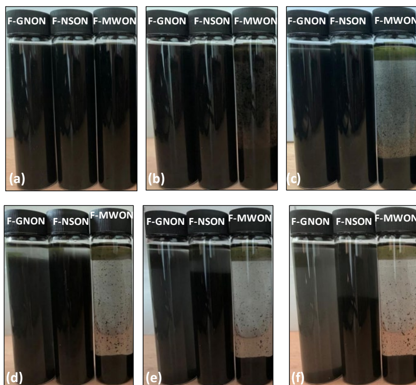
Figure 4. Dispersion stability test of fresh graphene-oil nanofluids after (a) completion of sonication, (b) one hour, (c) day-1, (d) day-3, (e) day-5 and (f) day-7 (arrangement from left: F-GNON, F-NSON and F-MWON) (Notes: F = fresh; H = heated) [40].
