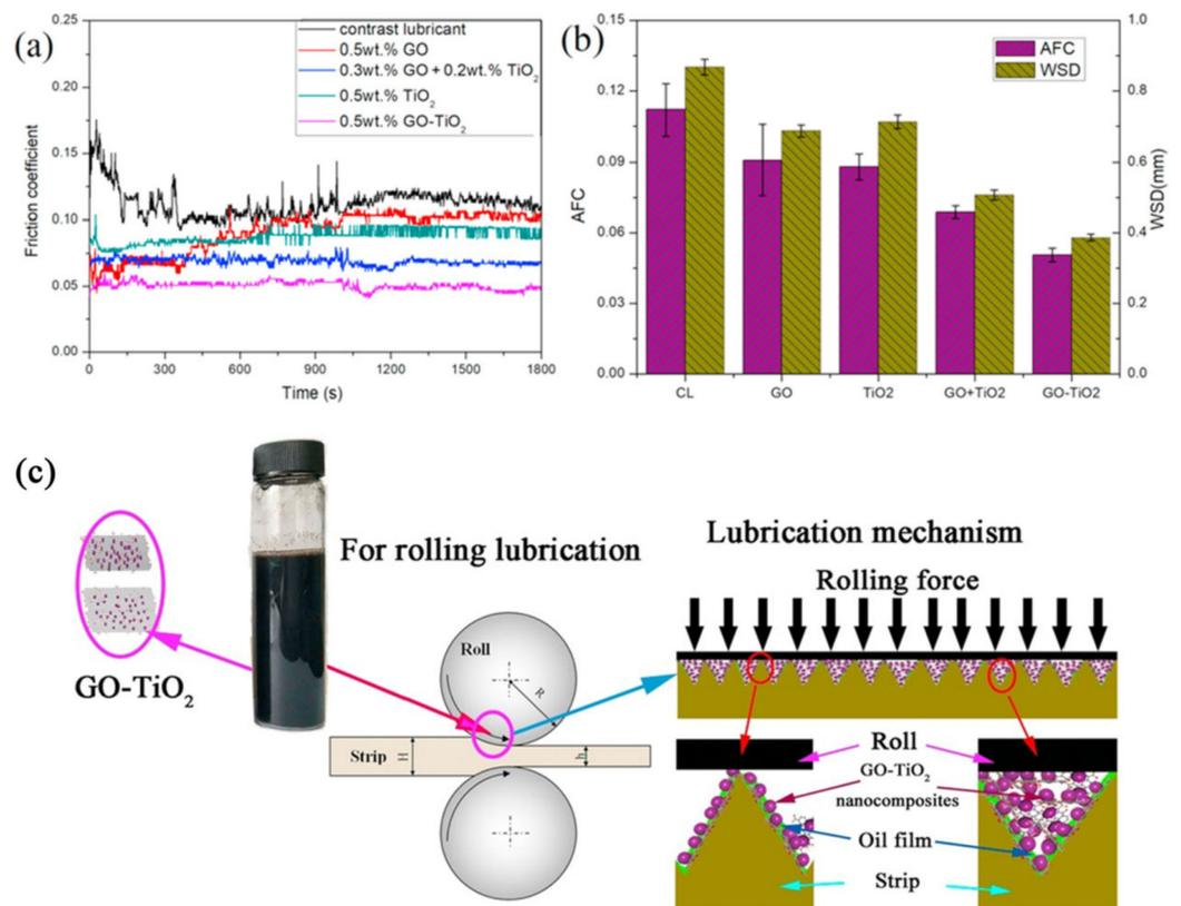
**Figure 12.** (a) COFs, (b) AFC and WSD of the wear scars lubricated by control group and GO, TiO<sub>2</sub>, GO+TiO<sub>2</sub>, and GO-TiO<sub>2</sub> nanofluids. (c) Schematic of GO-TiO<sub>2</sub> nanofluid rolling lubrication mechanism (adapted from [184]).
