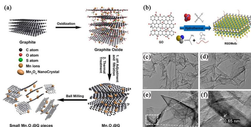
**Figure 2.** Synthetic process and structure of (a)  $Mn_3O_4$ @G (adapted from [45]), and (b) rGO/MoS<sub>2</sub> heterostructure. (c–f) Transmission electron microscopy (TEM) images of rGO/MoS<sub>2</sub> at different magnifications (adapted from [52]).
