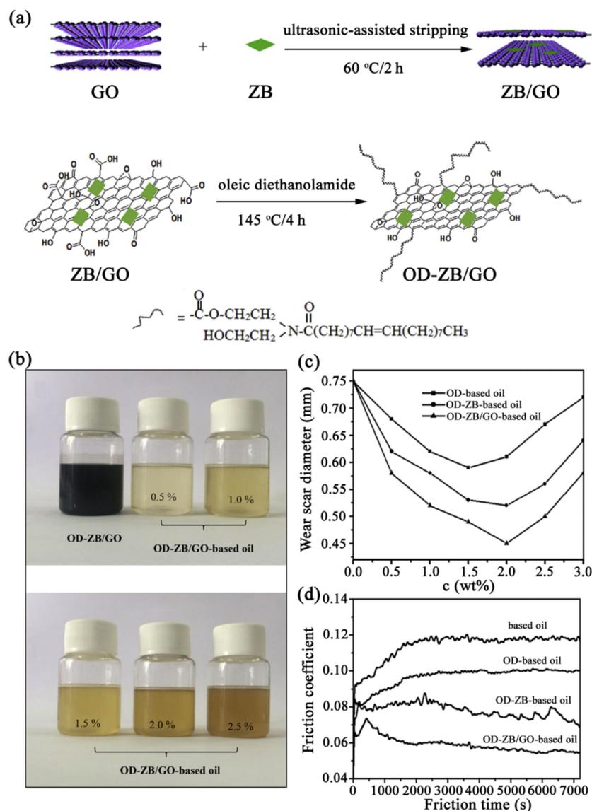
**Figure 11.** (a) The preparation and modification of ZB/GO. (b) Dispersion photos of OD-ZB/GO in the 500SN base oil with different contents. (c) The wear scar diameter (WSD) of the OD-based oil, the OD-ZB-based oil, and the OD-ZB/GO-based oil. (d) The friction coefficient curves of the 500SN base oil, the OD-based oil (2.0 wt%), the OD-ZB-based oil (2.0 wt%) and the OD-ZB/GO-based oil (2.0 wt%) (adapted from [178]).
