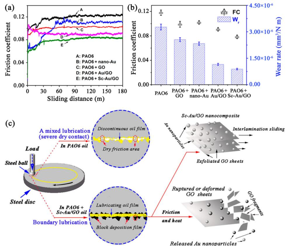
**Figure 10.** (a) COF curves of PAO 6 oil and PAO 6 oil containing different nanoparticles with 0.1 wt% (GO, nano-Au, Au/GO, and Sc-Au/GO). (b) Average COFs (FCs) and wear rates ( $W_{rs}$ ) of the corresponding discs lubricated with these oils. (c) Schematic of the lubricating models of PAO 6 oil and the Sc-Au/GO dispersed oil (adapted from [152]).
