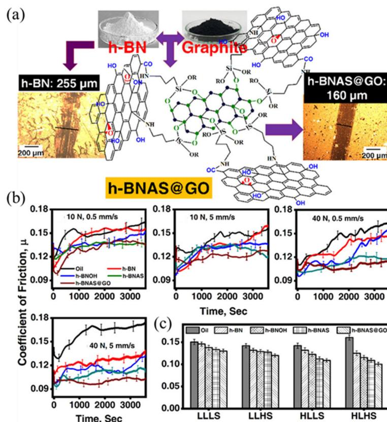
**Figure 9.** (a) Schematic diagram of the structure of the h-BNAS@GO composite material. (b) Variation in COF with sliding time from the ball loading macrotribometric studies for the prepared samples under different conditions. (c) Comparison of COF values (adapted from [145]).
