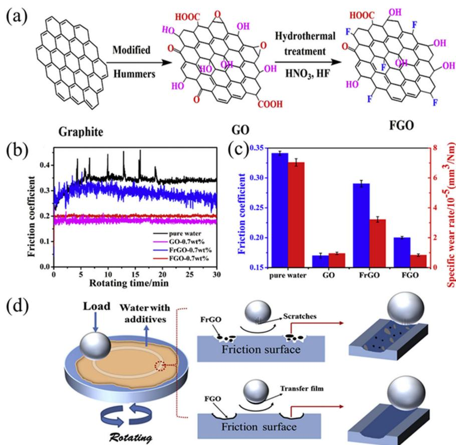
**Figure 5.** (a) Preparation of fluorinated graphene oxide. (b) COF and (c) wear rate for the water with GO-0.7 wt%, FrGO-0.7 wt%, and FGO-0.7 wt% at 5 N, 300 r/min, and duration of 30 min. (d) Friction mechanism model of water with FrGO and FGO additives (adapted from [94]).
