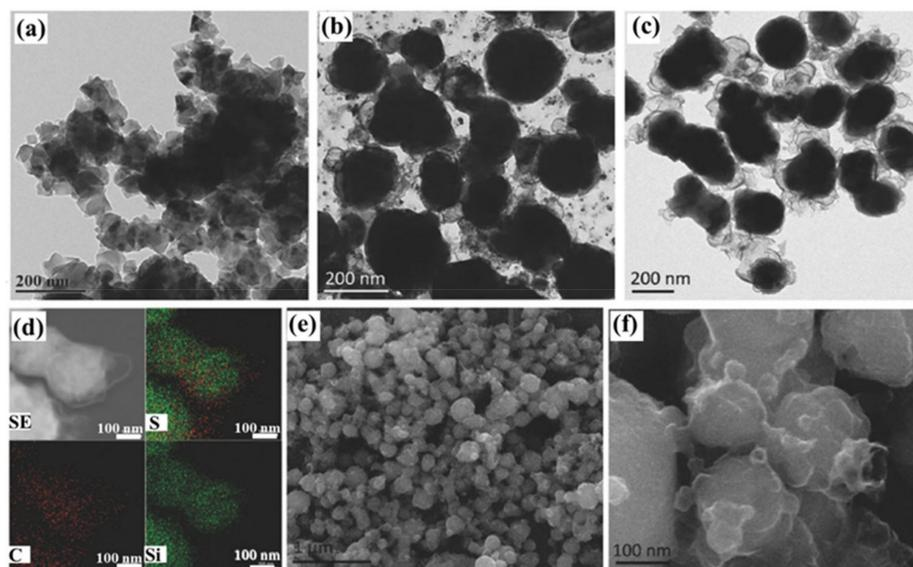
**Figure 3.** TEM images of (a) pristine SiC NPs, (b) SiC NPs irradiated by KrF pulsed laser, and (c) corresponding sample after washing. (d) Energy dispersive spectroscopy (EDS) elemental mapping of SiC@G. (e,f) Scanning electron microscopy (SEM) images of SiC@G after the acid etching and centrifugation (adapted from [54]).
