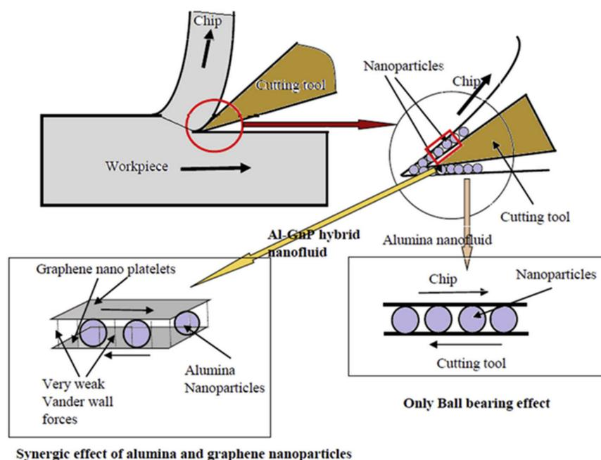
**Figure 13.** Synergic effect of alumina and Al-GnP nanoparticles trapped between the sliding surfaces (adapted from [149]).
