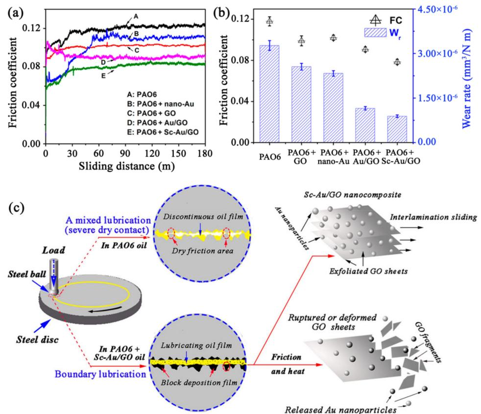
**Figure 10.** (a) COF curves of PAO 6 oil and PAO 6 oil containing different nanoparticle with 0.1 wt% (GO, nano-Au, Au/GO, and Sc-Au/GO). (b) Average COFs (FCs) and wear rates ( $W_{rs}$ ) of the corresponding discs lubricated with these oils. (c) Schematic of the lubricating models of PAO 6 oil and the Sc-Au/GO dispersed oil (adapted from [152]).
