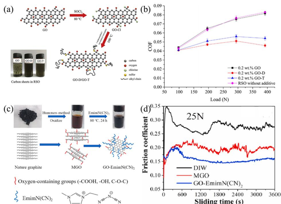
**Figure 7.** (a) Schematic illustration of synthesizing GO-D and GO-T. (b) Relationship between normal load and COF of GO, GO-D, and GO-T dispersions (adapted from [109]). (c) Preparation process of GO-EmimN(CN)<sub>2</sub>. (d) Friction curves of steel plates lubricated with pure water, 1.6 mg/mL MGO and GO-EmimN(CN)<sub>2</sub> dispersions at 25 N (adapted from [110]).
