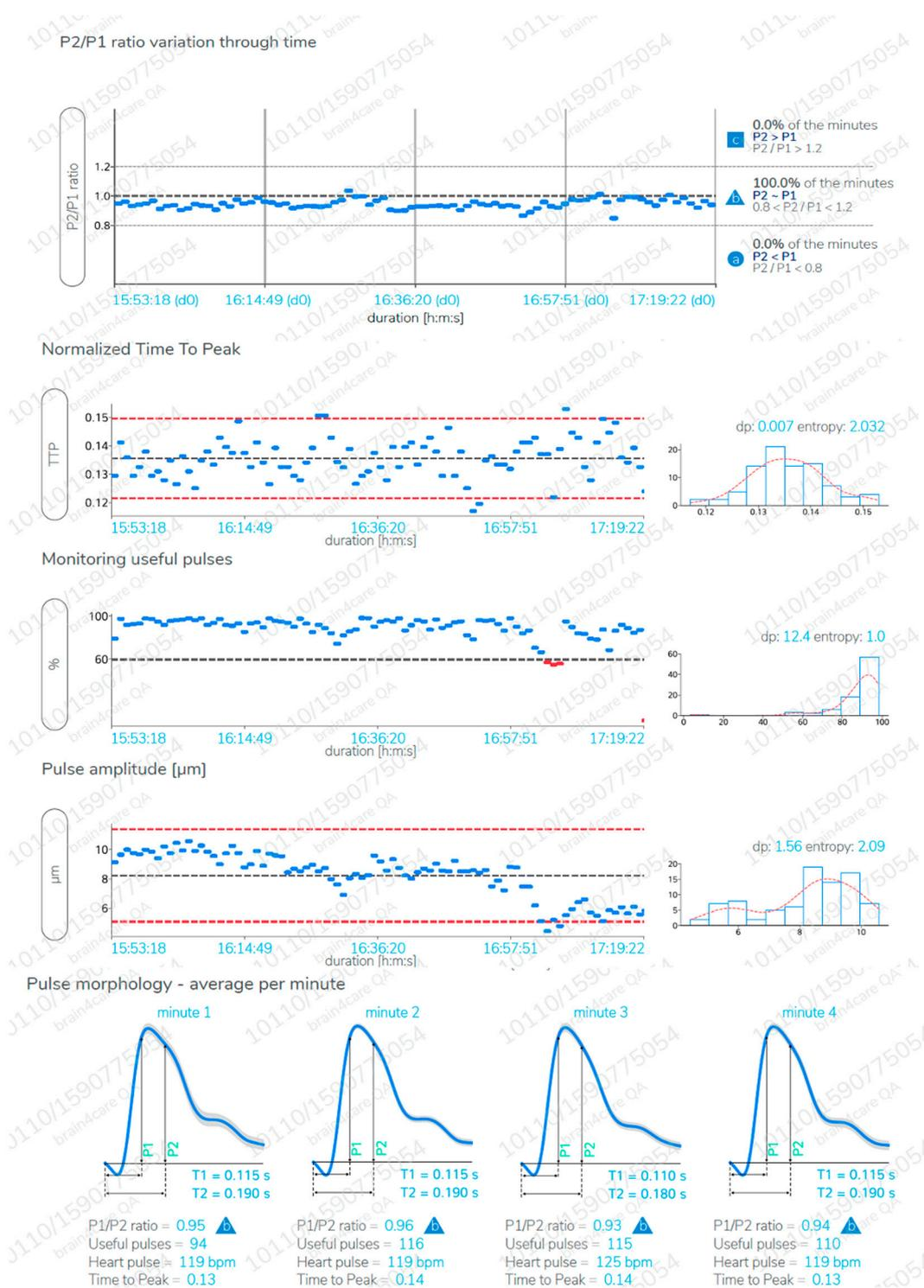
**Figure 3.** A B4C monitoring report sample of more than an hour length. Real time report is obtained without monitoring interruption as needed. P2/P1 ratio, time to peak, pulse amplitudes and useful pulses (pulses that were successfully recognized) are disclosed for the entire monitoring (each blue point is the mean value for a minute) and a mean waveform with confidence interval (gray zone along the slope) of each monitored minute is also displayed (bottom).
