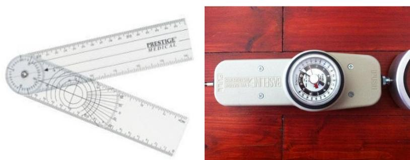
**Figure 3.** The standard analogue goniometer and baseline push–pull dynamometer used for the measurements.
