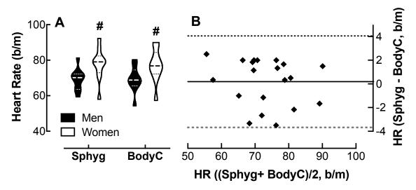
**Figure 2.** Comparison of heart rate (HR measured by the Body Cardio with SphygmoCor determinations. (**A**) Violin plot of HR measured by the Sphyg and BodyC in men and women; p < 0.01, male vs. female by two-way ANOVA; n = 10/group. (**B**) Q-Q plot of HR determined by the Sphyg and BodyC. Each data point represents duplicate or triplicate measures in one study participant. HR, heart rate.
