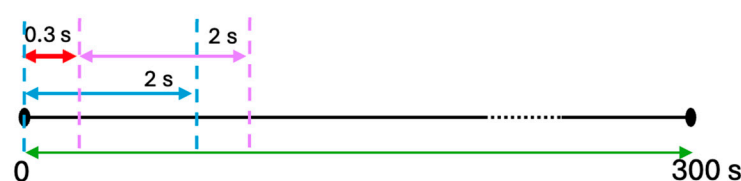
Figure 4. Training trials creation using an overlapping window; the red arrow represents the stride.
