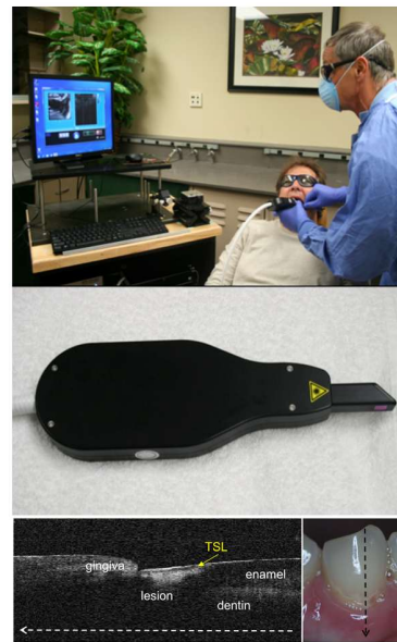
Figure 3. Clinical OCT system and handheld 2D scanner, along with a CP-OCT image of an arrested lesion on the tooth buccal surface acquired in vivo. The CP-OCT b-scan matches the position of the dashed arrow. The dark band of reduced reflectivity near the surface of the lesion is the TSL. From reference [53].
