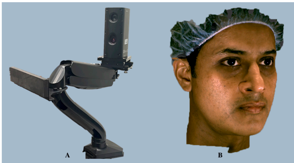
Figure 6. Accu3D facial imaging system (A) and an automatically merged 3D facial scan generated using the Accu3D face acquisition system (B).
