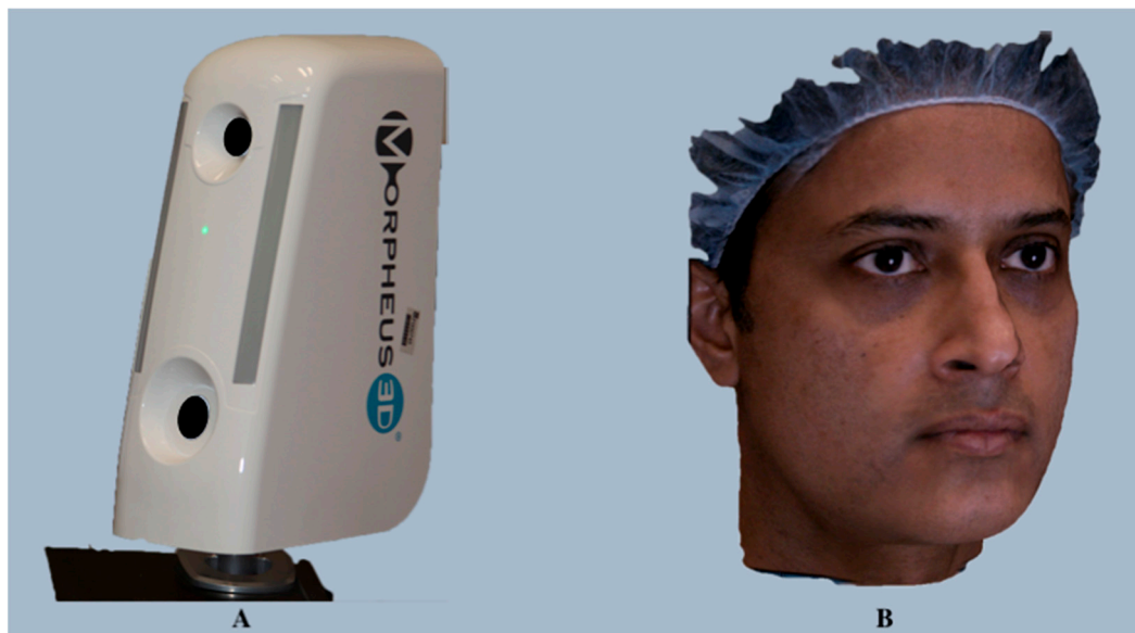
Figure 5. Morpheus 3D facial imaging system (A) and a sample of a single composite 3D facial image generated using the Morpheus 3D face acquisition system (B).
