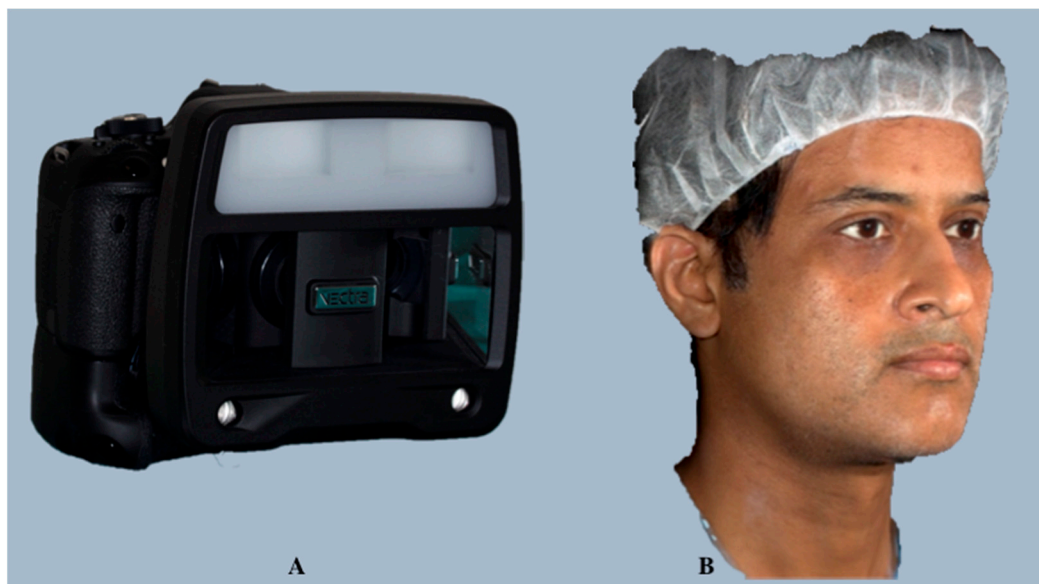
Figure 4. Vectra H1 facial imaging system (A) and an automatedly stitched 3D facial scan generated using the Vectra H1 face acquisition system (B).
