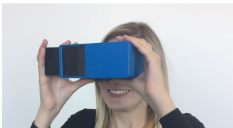
Figure 1. Demonstration of use of the box apparatus. The smartphone inserts into the box from the side (Mariakakis et al. [30]).
