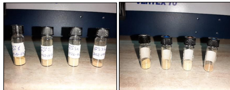
Figure 3. GSs ground in a mortar used for FTIR analysis.
