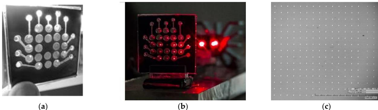
**Figure 5.** Experimental assembly of the matrix chip (a); a matrix chip in the installation illuminated by laser beams transmitted through the grating (b); and a micrograph of the diffraction grating from anodic alumina (c), where the window diameter is 10  $\mu\text{m}$  and the distance between the windows is 100  $\mu\text{m}$ .
