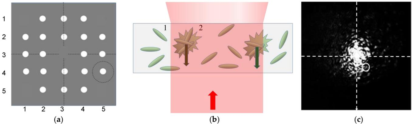
**Figure 11.** Registration of suspensions of microorganisms in a matrix chip using a 2D collimator (a) for the array of 20 measuring cuvettes, an optical scheme of the speckle excitation in microcells (b), where 1—microorganism, 2—cluster of microorganisms, and the speckle field of the cuvette of the *E. coli* M-17 filled in phosphate buffer (c), where the white circle indicates the signal reception aperture.
