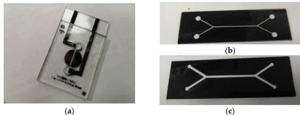
**Figure 4.** Sample capillary chips for LLS measurements: capillary ( $H \times W \times L$ ) 0.1 mm  $\times$  1 mm  $\times$  10 mm (a); 0.08 mm  $\times$  0.7 mm  $\times$  30 mm (b); and 0.08 mm  $\times$  1.5 mm  $\times$  30 mm (c).
