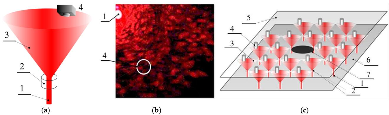
**Figure 3.** Schematic presentation of the principle of positioning of the detector unit (a,b) and multi-channel ABR detection scheme using split laser beam (c). 1—laser beam,  $\lambda = 645$  nm; 2—scattering volume; 3—scattered light field; 4—pin-photodiode; 5—cover of the multichannel chip; 6—base; and 7—shutter.
