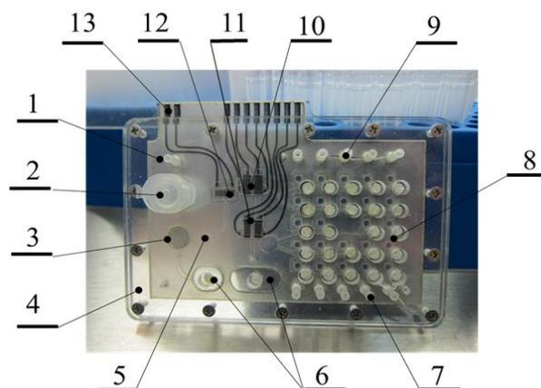
**Figure 1.** A sample model of lab-on-a-chip for total microbiological analysis. 1—pump inlet; 2—swab inlet well; 3—growth chamber; 4—case; 5—CCD image capture area; 6—waste basins; 7, 9—antibiotic injection sleeves; 8—bacteria viability testing cells (two series of 10 cells); 10—impedimetric sensor; 11—SAW keys; 12—acoustic sensor; and 13—contact pads [9].
