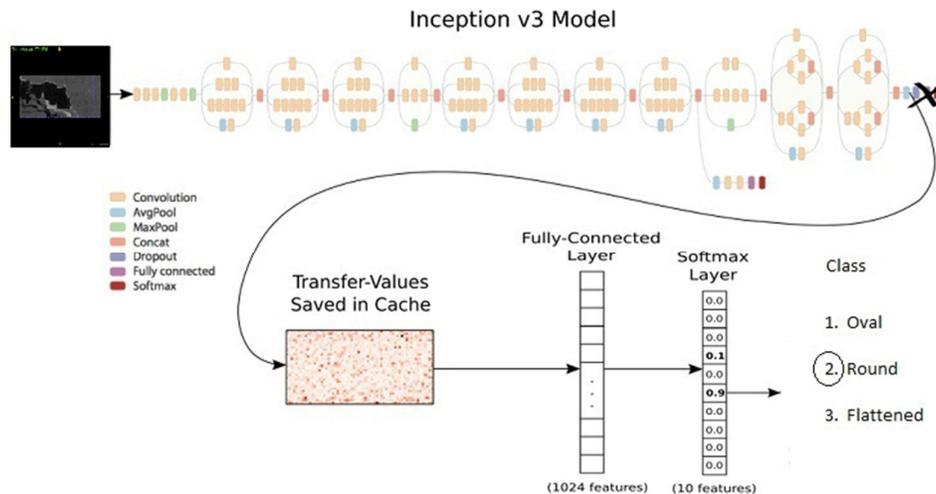
**Figure 4.** Deep CNN architecture of automatic sella classification.
