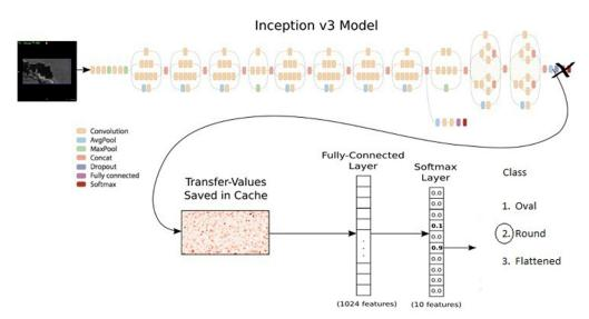
Figure 4. Deep CNN architecture of automatic sella classification.
